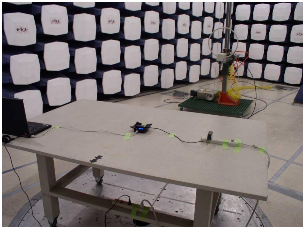
**Radiated Emission above 30MHz – Front View**
