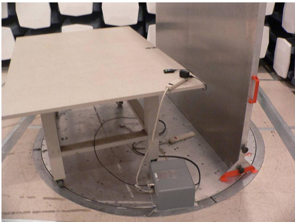
**Radiated Emission below 30MHz – Front View**
