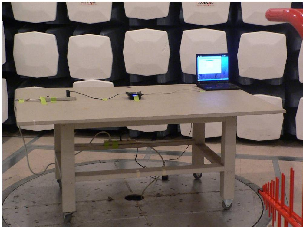
**Radiated Emission above 30MHz – Rear View**
