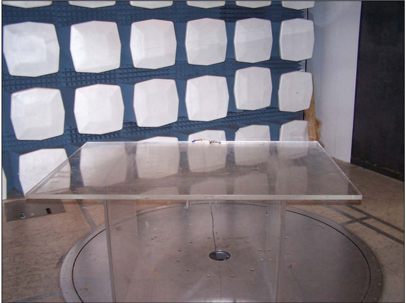
Photograph 2. Radiated Emissions Limits, Test Setup
