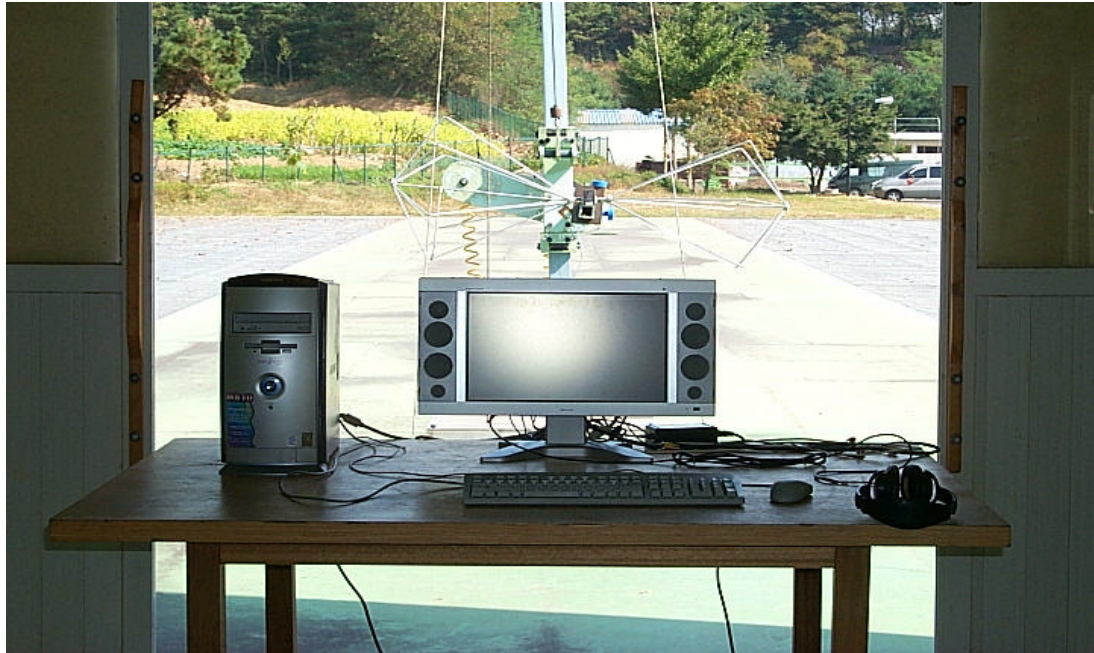
Photograph 2 : Setup for Radiated Emissions
