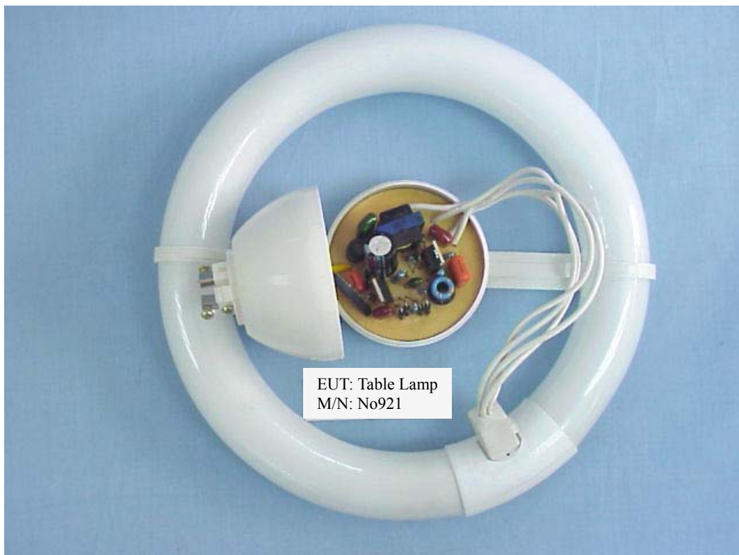
FIGURE 2 TABLE LAMP (M/N: No921) COVER REMOVED#1 (BALLAST M/N KFE-C22W)
