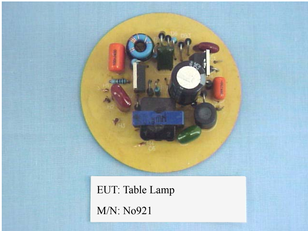
FIGURE 4 TABLE LAMP (M/N: No921) MAIN BOARD: COMPONENT SIDE (BALLAST M/N KFE-C22W)
