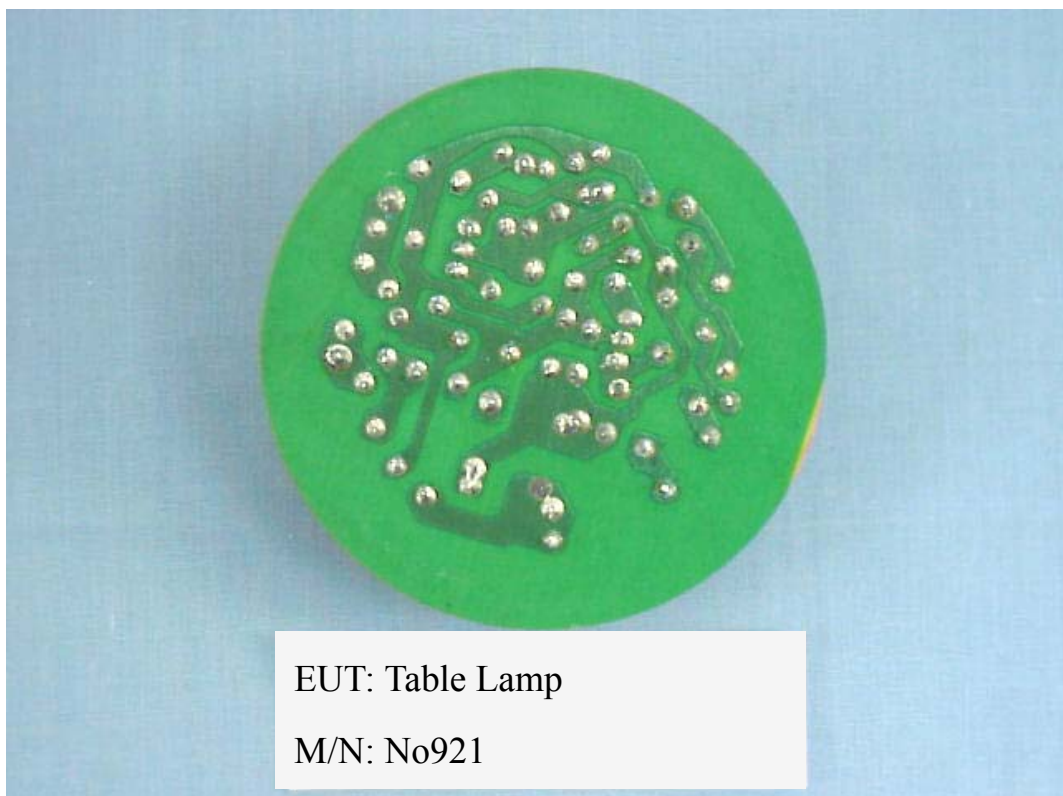
FIGURE 5 TABLE LAMP (M/N: No921) MAIN BOARD: SOLDERED SIDE (BALLAST M/N KFE-C22W)
