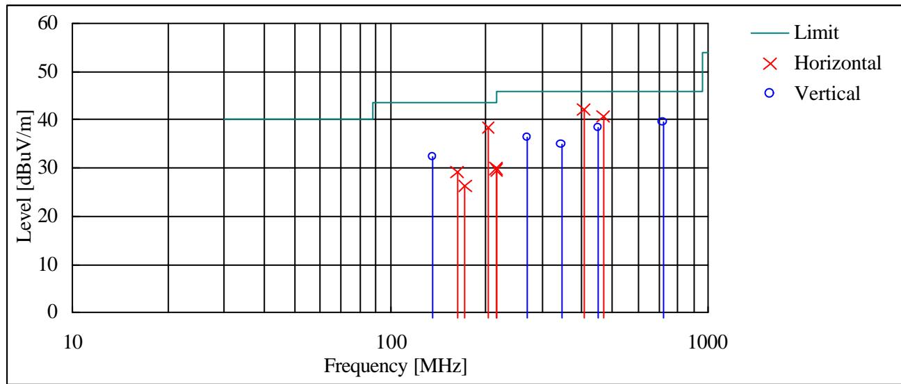
Notes: The test is performed in a distance of 3m. Af : Antenna factor, Cl : Cable loss
