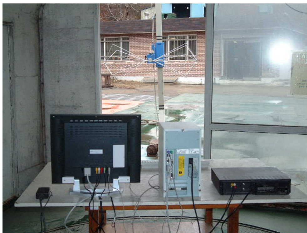
RADIATED EMISSION SETUP PHOTOGRAPH - REAR VIEW ( 30 - 300 MHz )
