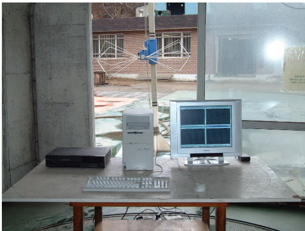
RADIATED EMISSION SETUP PHOTOGRAPH - FRONT VIEW ( 30 - 300 MHz )
