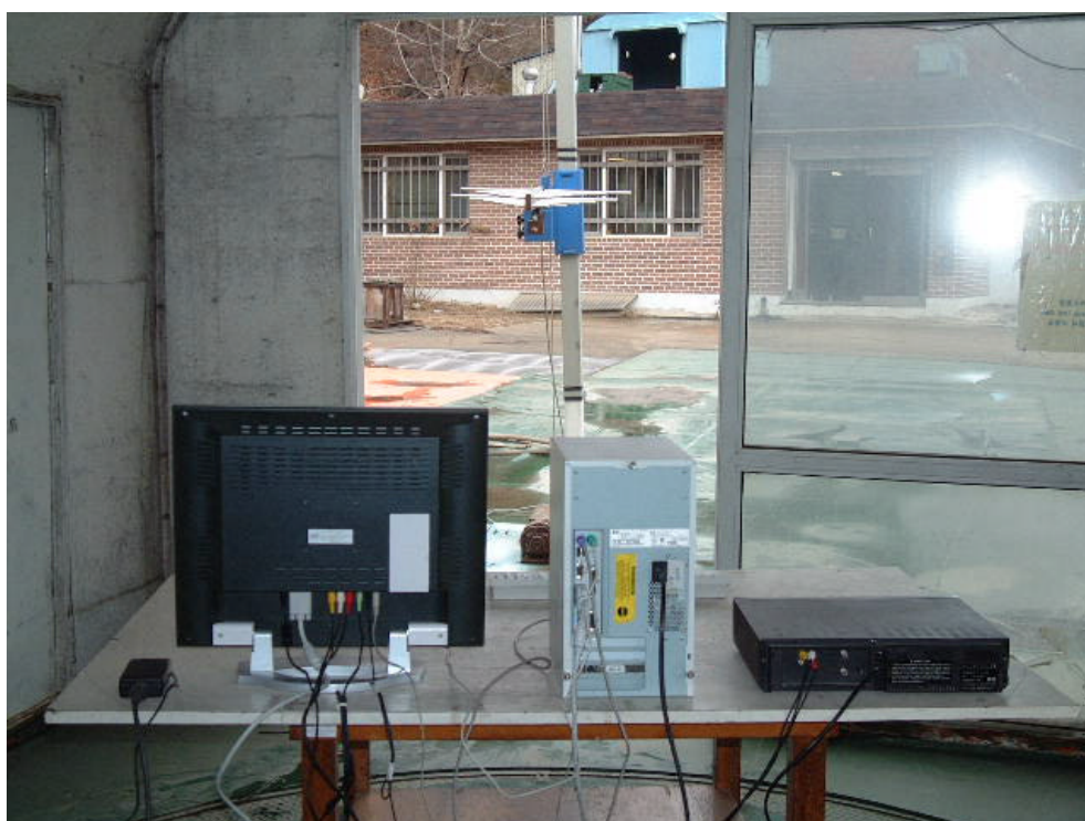
RADIATED EMISSION SETUP PHOTOGRAPH - REAR VIEW ( 300 - 1000 MHz )
