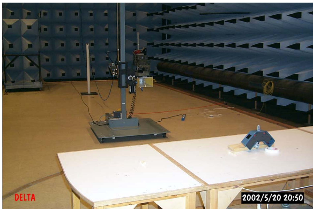
Photo 2 Set-up for measurements 1 GHz to 10 GHz.
