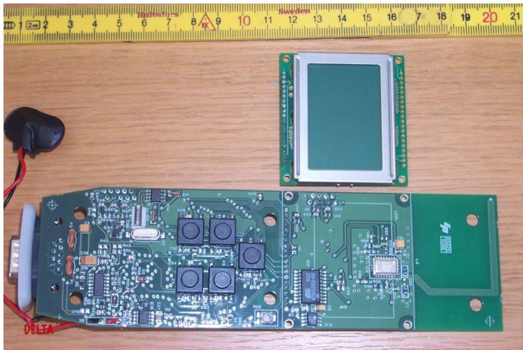
The display module shown next to the main board will be mounted on top of the board, on the same side as the push buttons, fixed by four screws. Measurements in cm.
