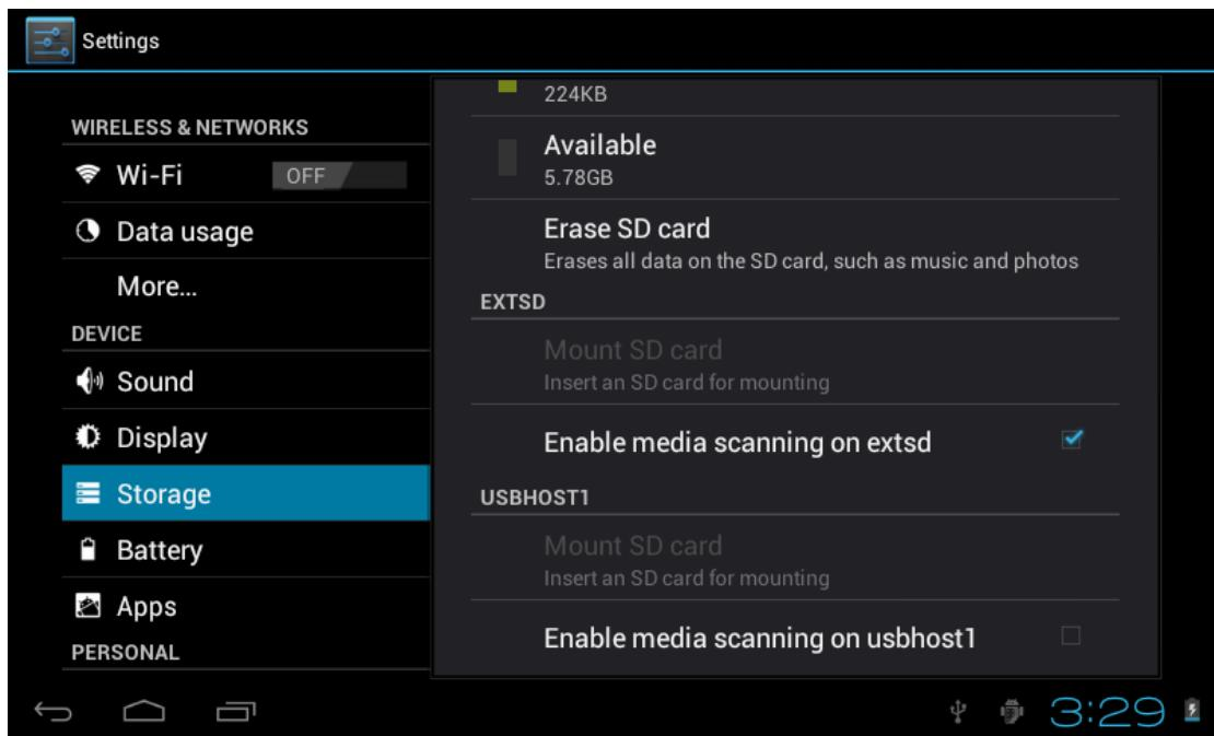
【Remark】: pls touch option "delete SD card", so that can safety to remove SD card
