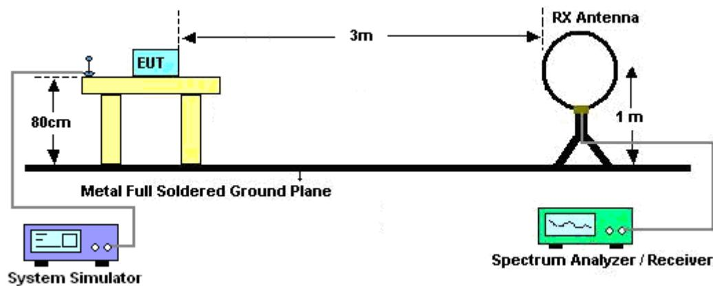
For radiated emissions from 30MHz to 1GHz
