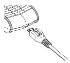
Insert the charger connector into the bottom of your Vertu phone as shown. Please ensure that the connector is inserted correctly, with the connector symbol uppermost.
