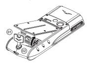
With the back of your Vertu phone facing you, position the back cover release key (01) into the slot of the locking screw (02).
