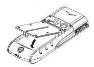
To replace the back cover, locate the internal clip (06) first.
