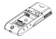
Slide the locking mechanism (04) over the SIM card to hold it in place.
