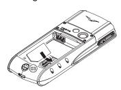
Insert the SIM card into the SIM card compartment, ensuring that the bevelled corner (03) is located bottom right and the gold contact area is facing downwards.
