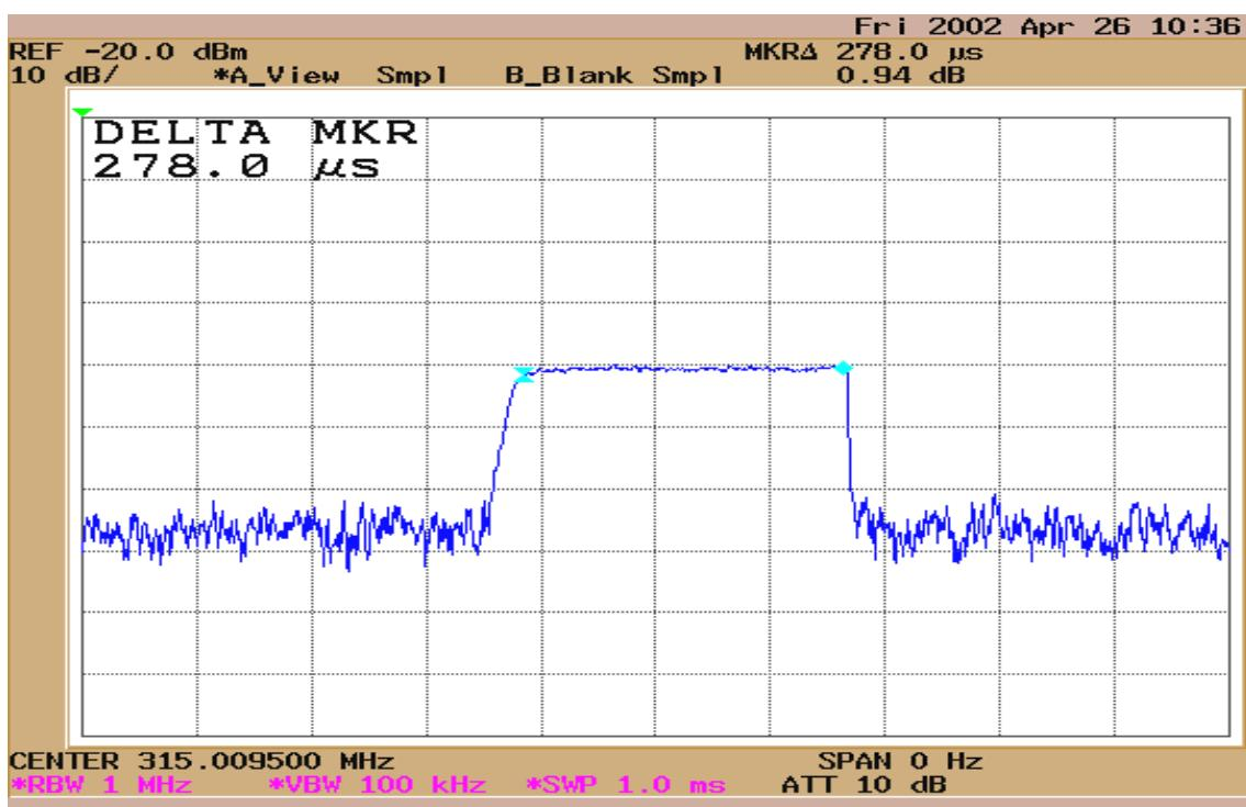
the transmitter operation is completed within 5seconds
