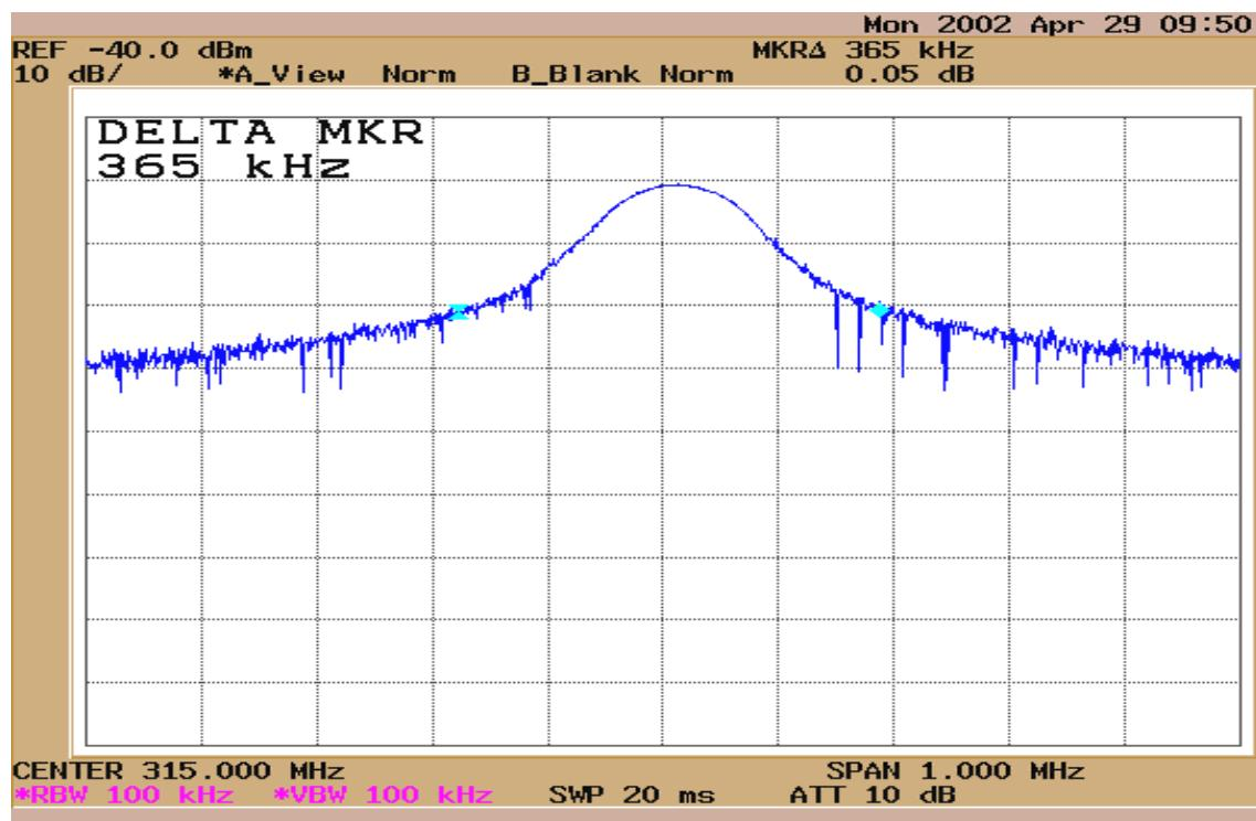
the bandwidth of the emission at the 20dB point is 365KHz
