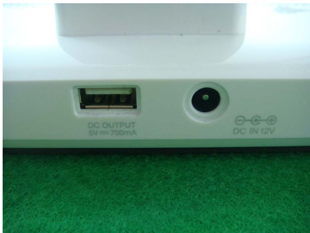
<Photograph 8: Rear View (DC jack(DC 12 V input), USB(DC 5 V output))>
