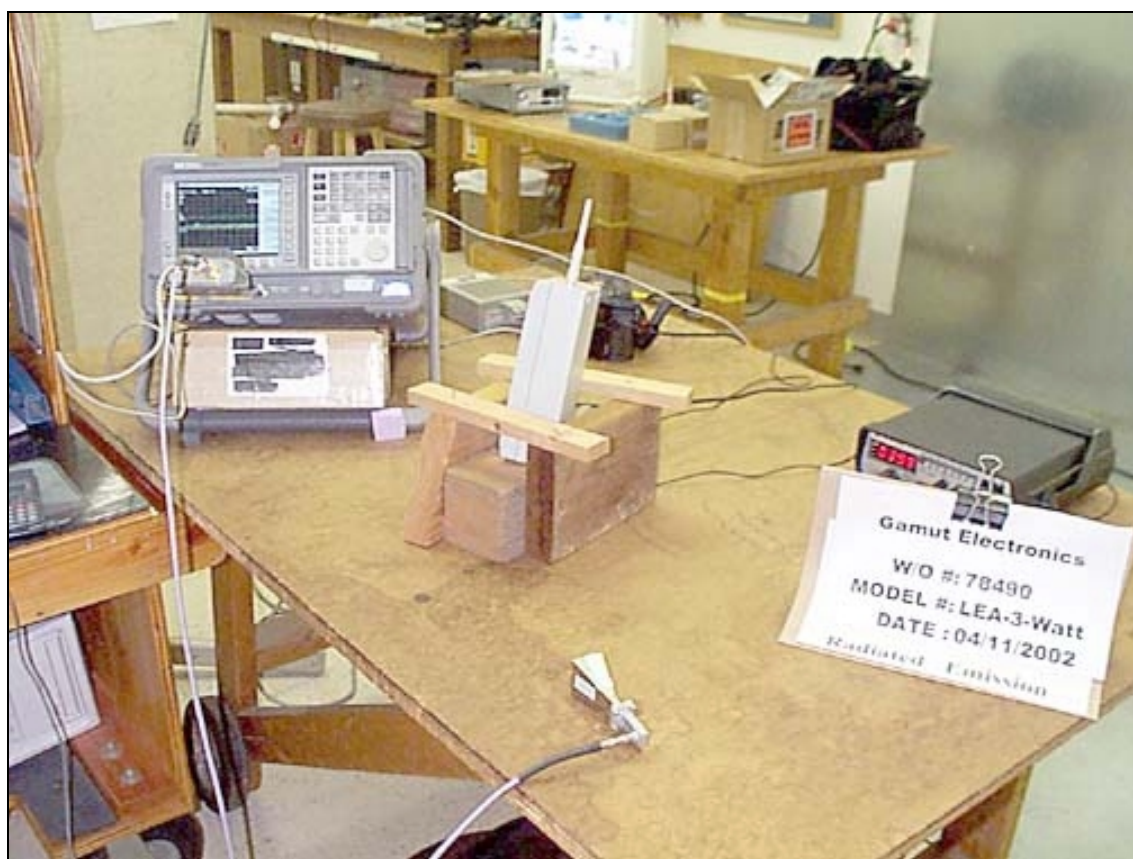
OATS Test Setup - Horn Antenna
