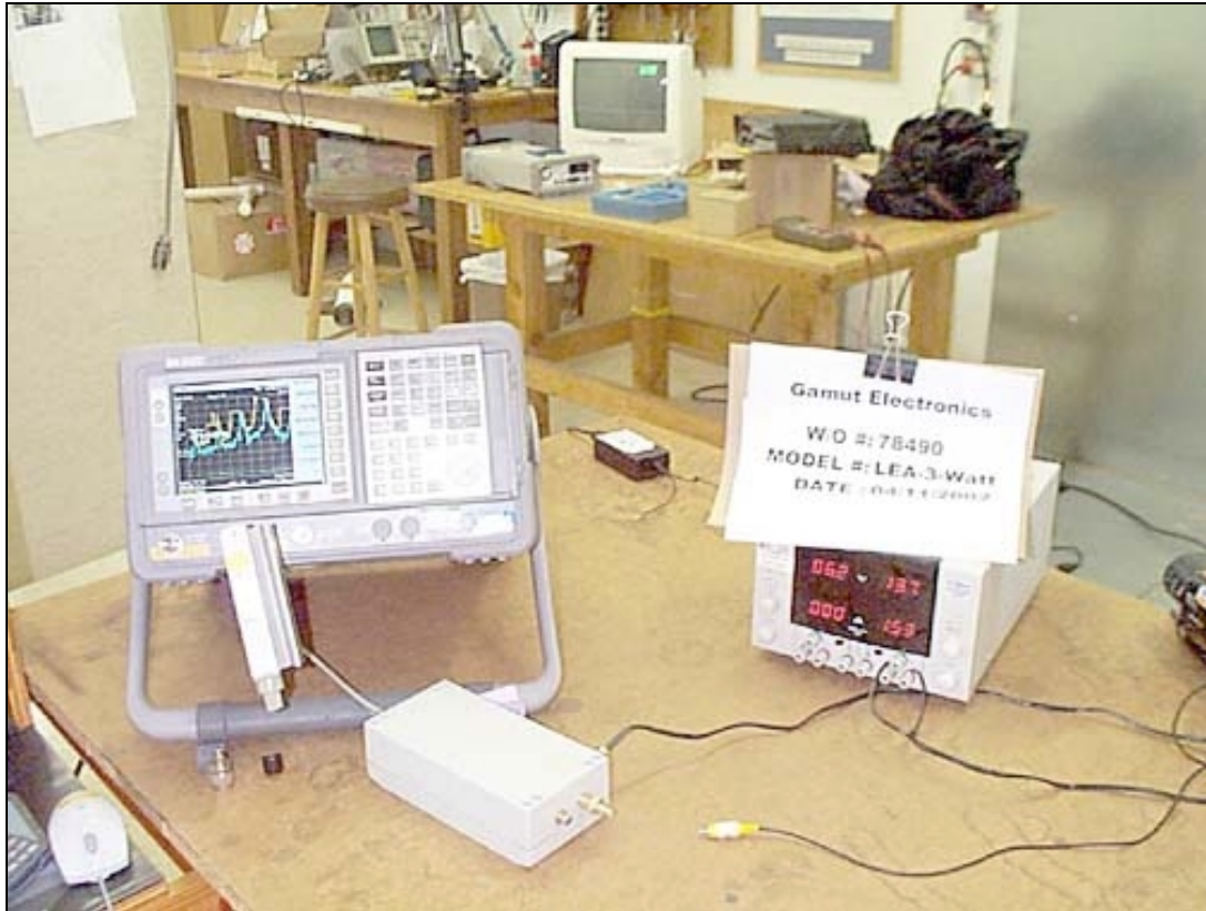
Voltage Variations Test Setup
