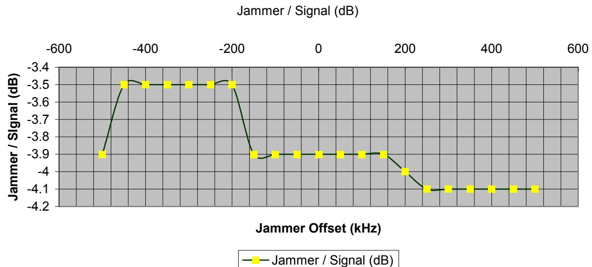
**TEST RESULTS****FCC Part 15C (15.247(d)(2)) Processing Gain (Direct Sequence System) Results**
