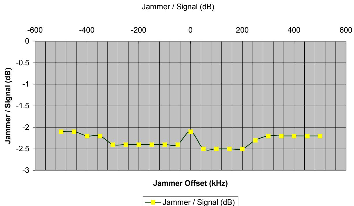
FCC Part 15C (15.247(d)(2)) Processing Gain (Direct Sequence System) Results
