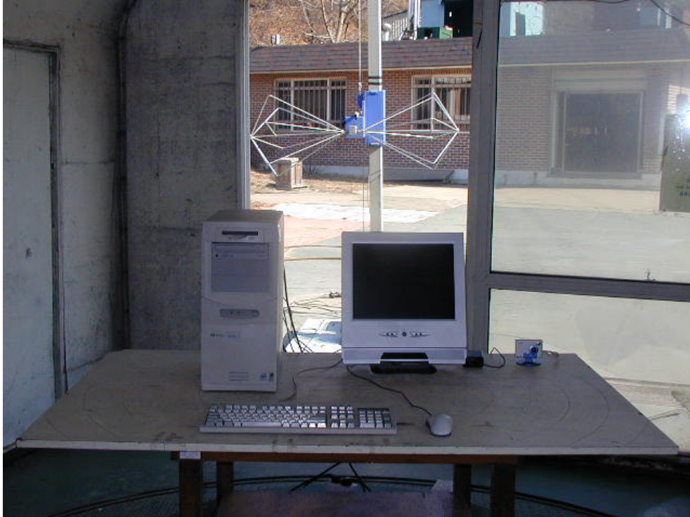
RADIATED EMISSION SETUP PHOTOGRAPH - FRONT VIEW ( 30 - 300 MHz )
