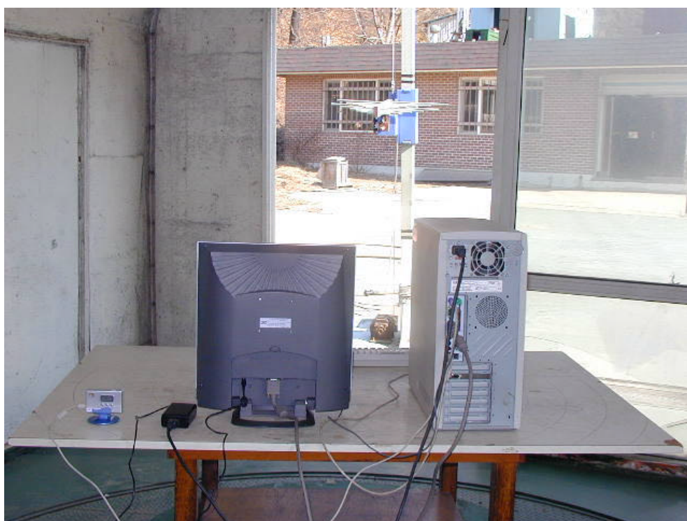
RADIATED EMISSION SETUP PHOTOGRAPH - REAR VIEW ( 300 - 1000 MHz )
