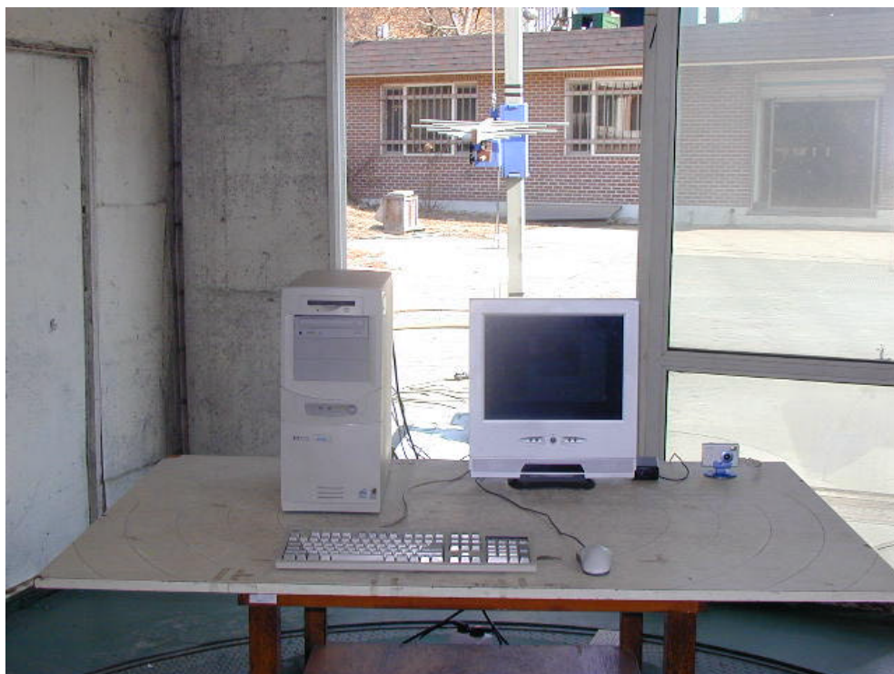
RADIATED EMISSION SETUP PHOTOGRAPH - FRONT VIEW ( 300- 1000 MHz )
