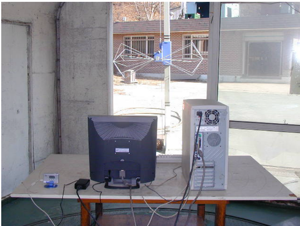
RADIATED EMISSION SETUP PHOTOGRAPH - REAR VIEW ( 30 - 300 MHz )
