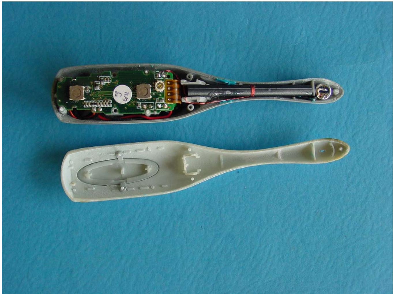
Photo 4. Headset: Printed circuit board: switches side
