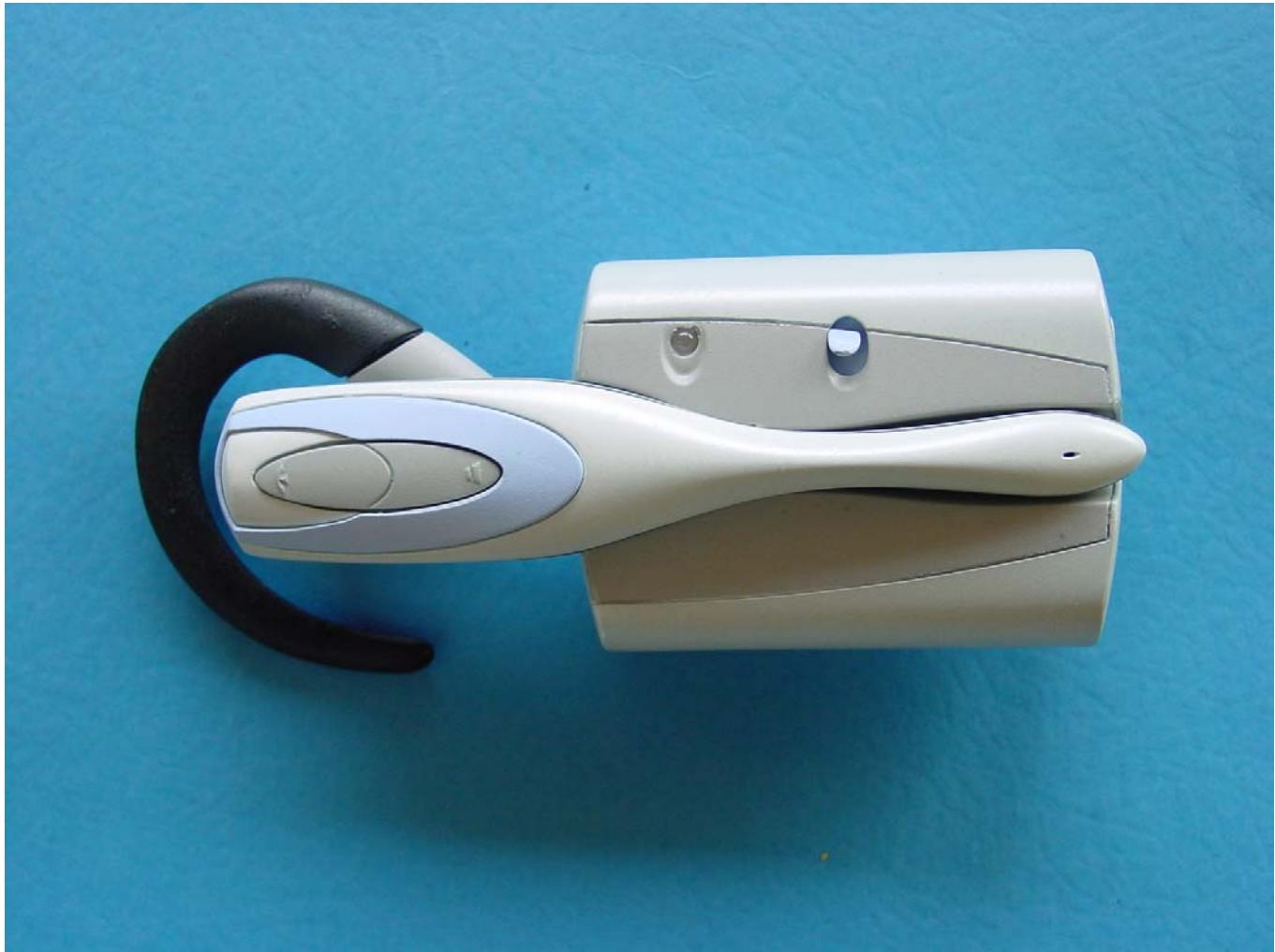
Photo 1. Wireless Headset System: Base unit & Headset in the charge mode
