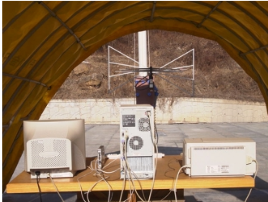
Photograph 1 : Setup for radiated Emissions
