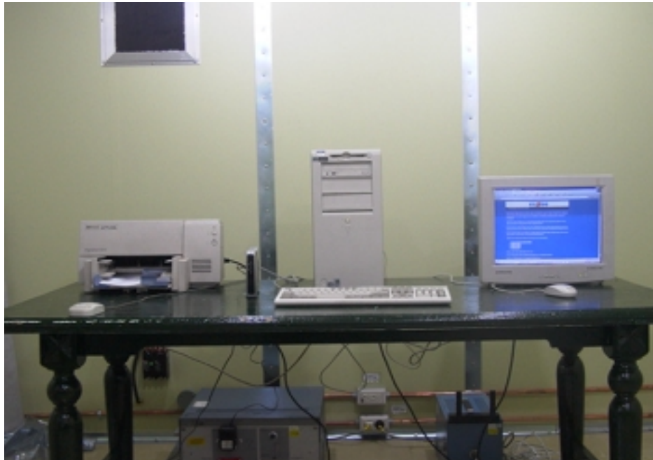
Photograph 2 : Setup for Conducted Emissions
