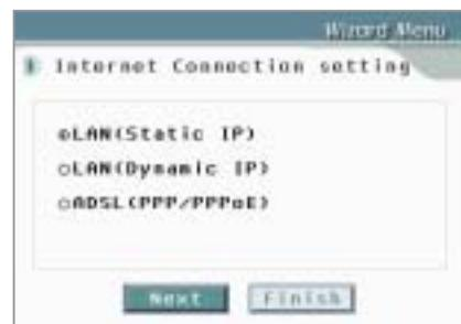
**NOTE.** When connecting the IP Videophone to LAN or the cable network, select 'LAN(Static IP)' if the address of the IP Videophone is already fixed, or select 'LAN(Dynamic IP)' if the IP address is dynamically allocated. If you have subscribed to the ADSL network, select 'ADSL (PPP/PPPoE)'.
