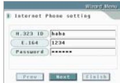
**NOTE.** Because the IP Videophone conforms to H.323 international video communication standard, you can register the unit to the Internet phone service. In order to connect the phone to the Internet phone service network, you should set the H.323 ID to be used in the server address and authentication process, and the ID in the format
