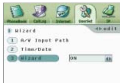
**NOTE.** If the Wizard is set to 'ON', the wizard menu is started when the system is rebooted. Once the wizard function is used, it is automatically set to 'OFF'.
