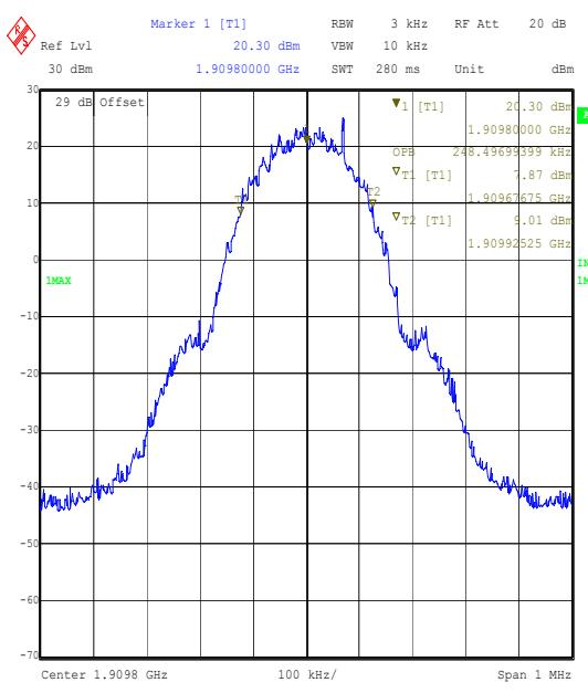
*Note: The occupied bandwidth is measured using the internal OBW function of the measurement analyser. The analyser automatically configures the measurement bandwidths to make an accurate measurement. The vital data is reported in the upper right portion of the screen. See attached graphs.*
