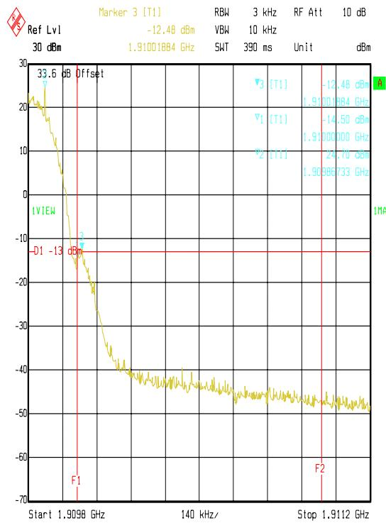
**Transmitter Out of Band Radiated Emissions (Band Edge): Section 2.1051/24.238 (Continued)**
