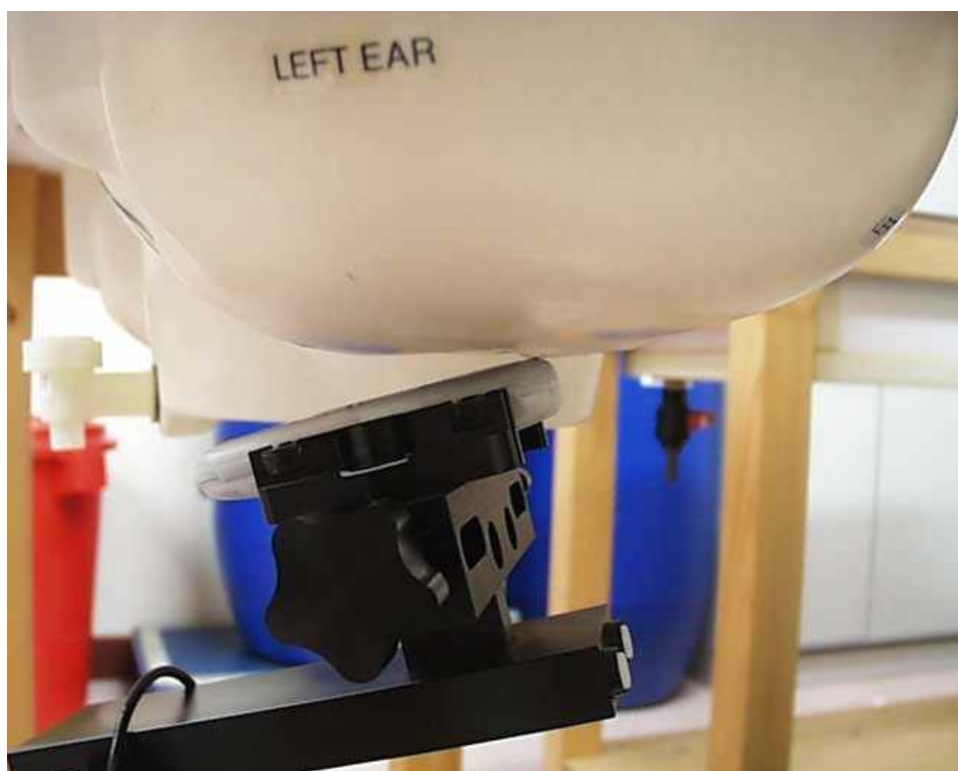
SAR Test Setup (Device at Head Phantom) – Closer Side View (Ear/Tilt)
