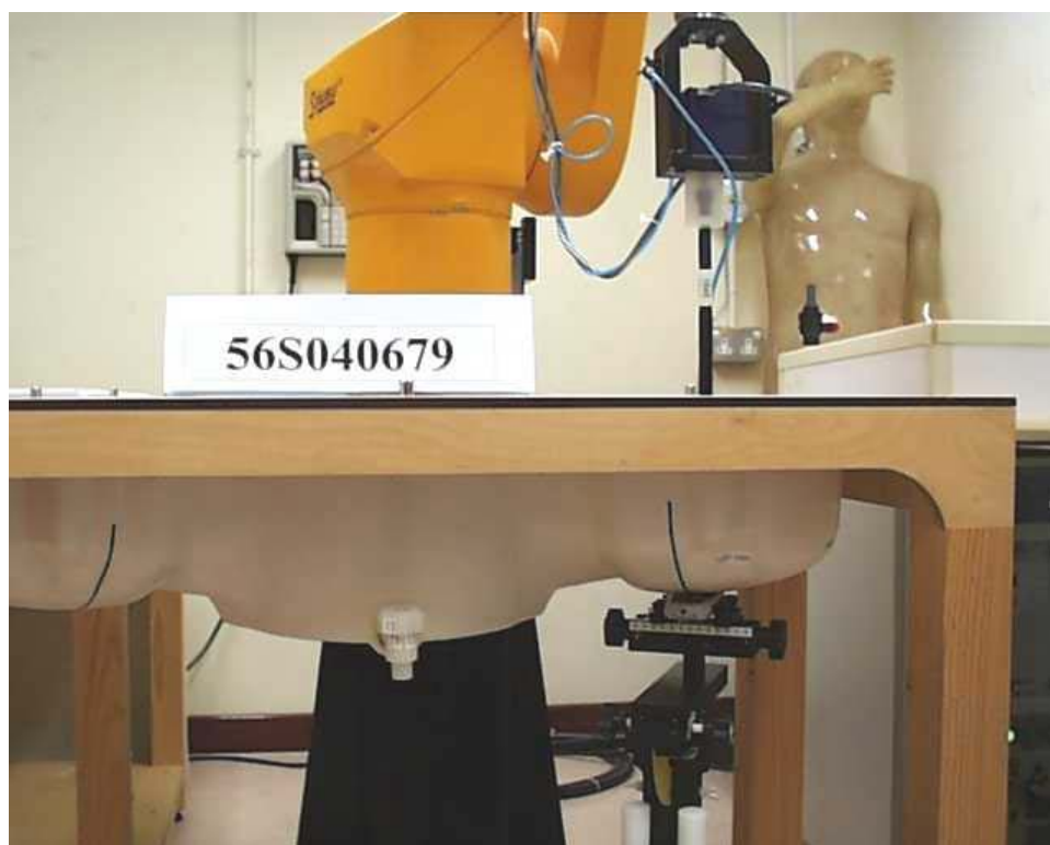
SAR Test Setup (Device at Head Phantom)
