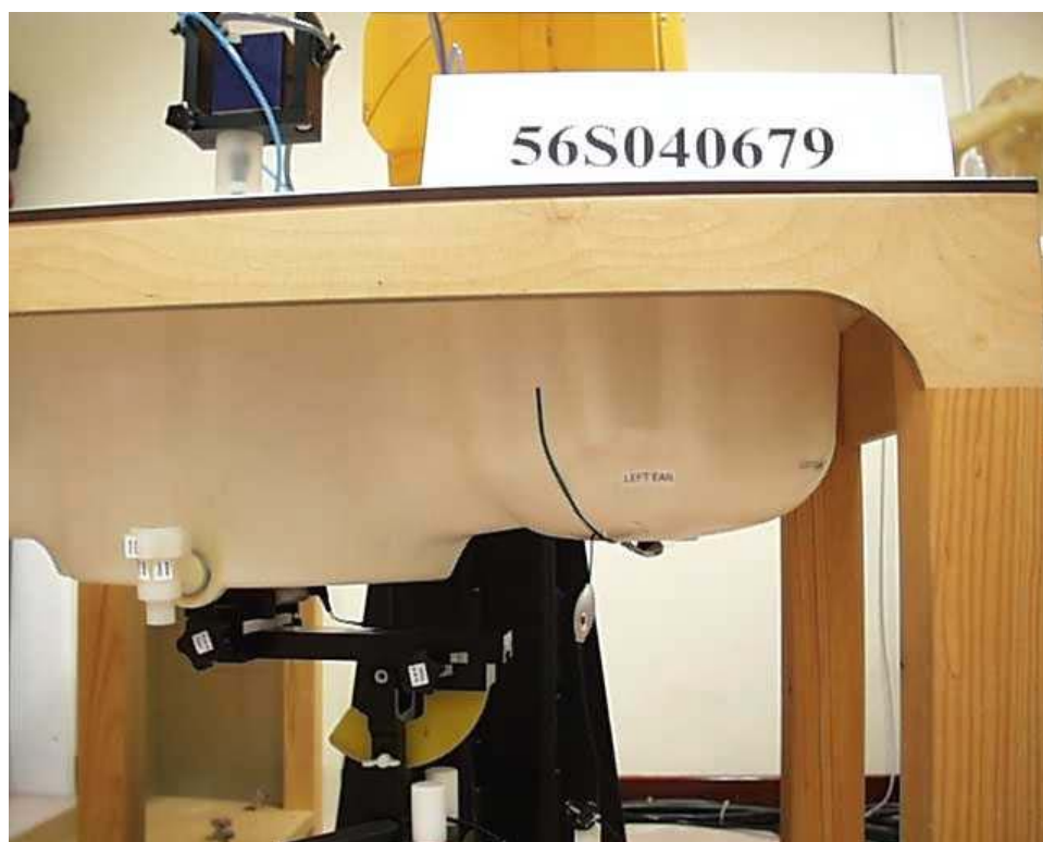
SAR Test Setup At Flat Phantom
