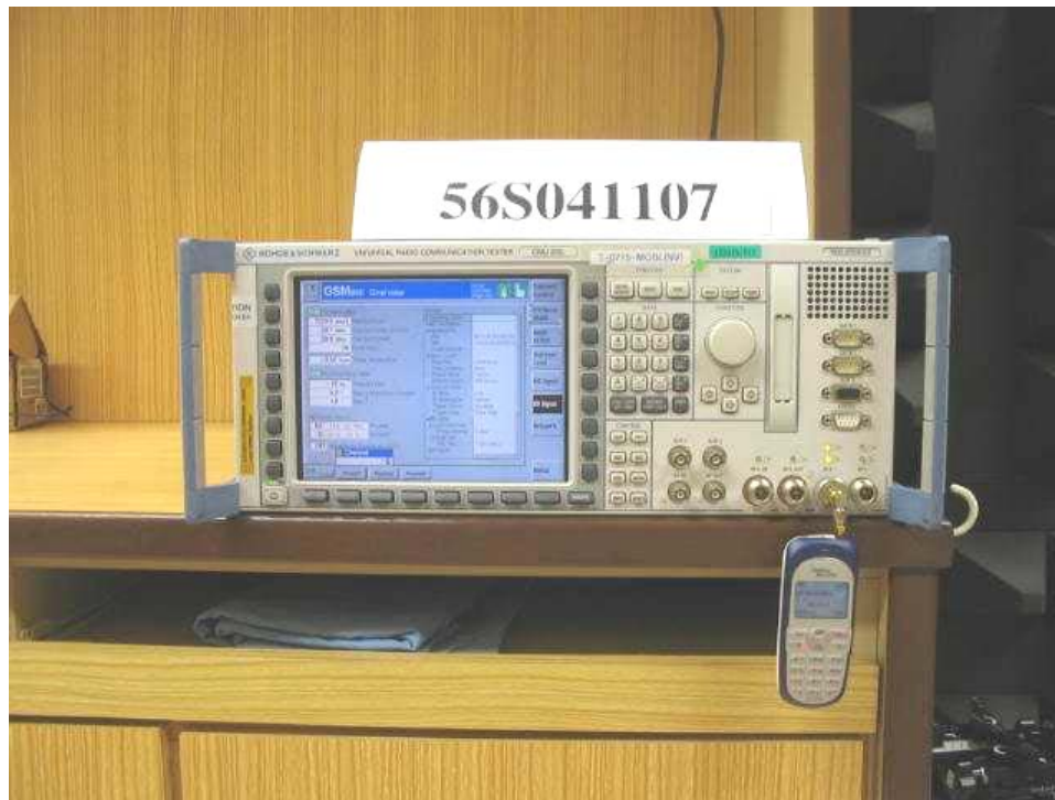
Conducted Power Measurement Setup – Far View
