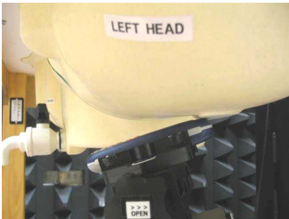
SAR Test Setup (Device at Head Phantom) – Closer Side View (Ear/Tilt)
