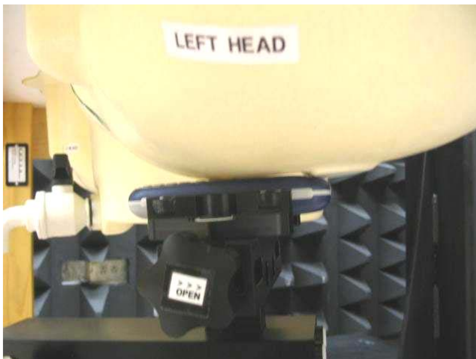
SAR Test Setup (Device at Head Phantom) – Closer Side View (Cheek/Touch)
