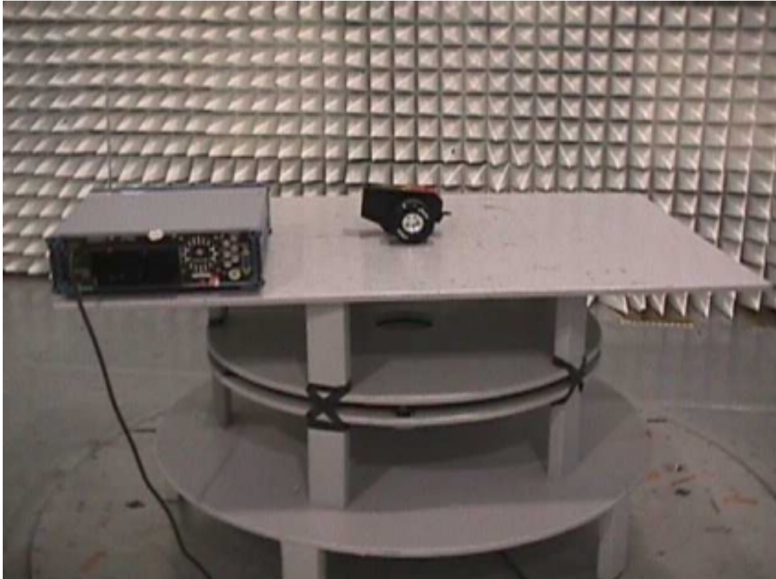
Radiated Emissions Test Configuration
