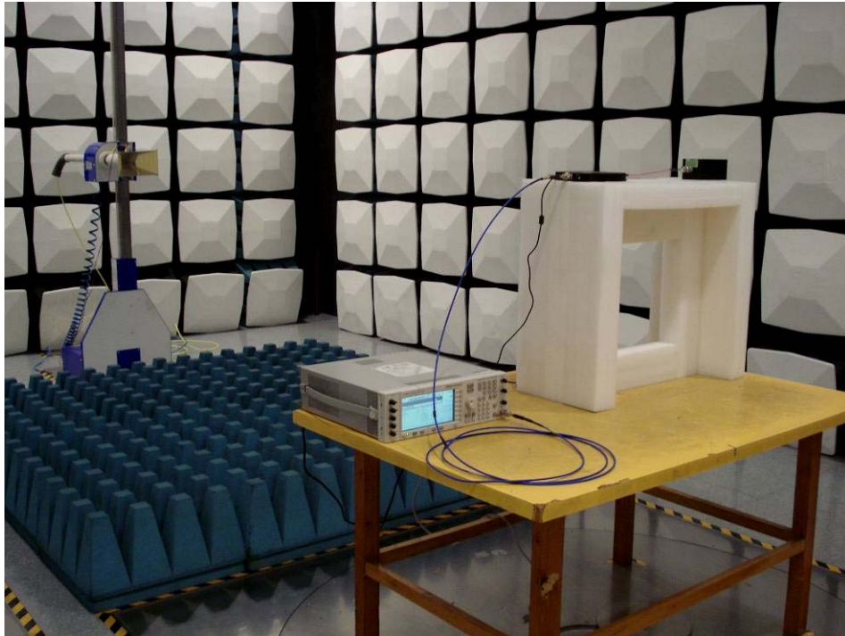
Spurious Emissions Test Setup - Rear View
