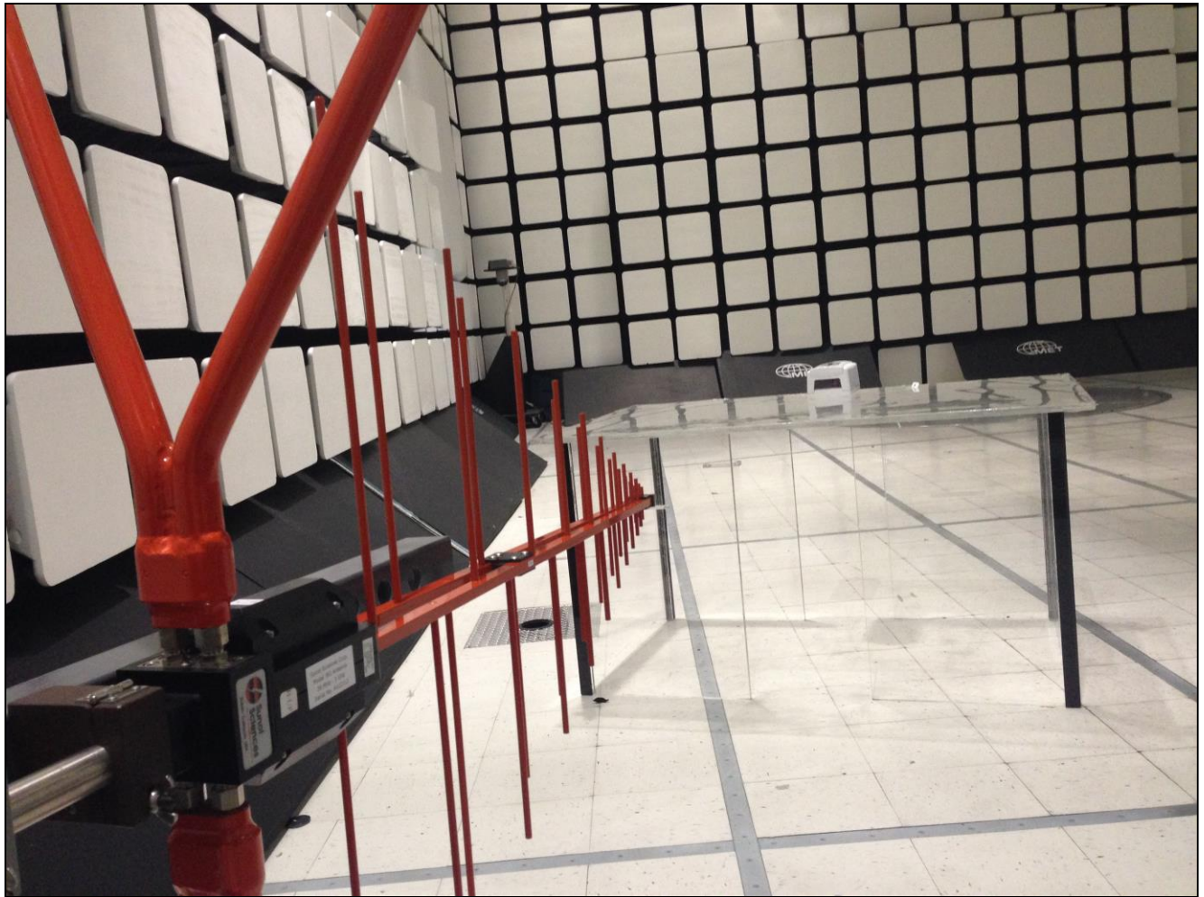
Photograph 4. Fundamental Field Strength, Harmonic/Spurious Emissions, 30 MHz – 1 GHz, Test Setup
