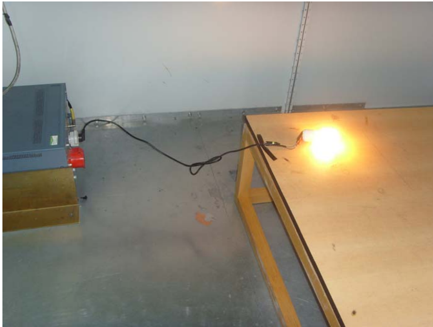
Conducted Emissions Test Set-up
