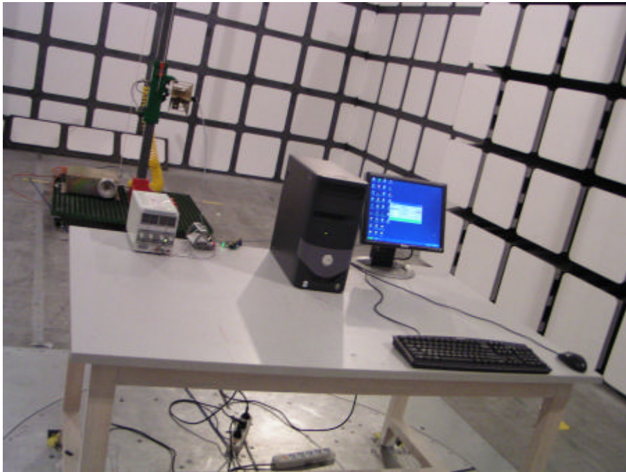
Transmitting Mode: Radiated Emission – Rear View (1000-25000MHz)
