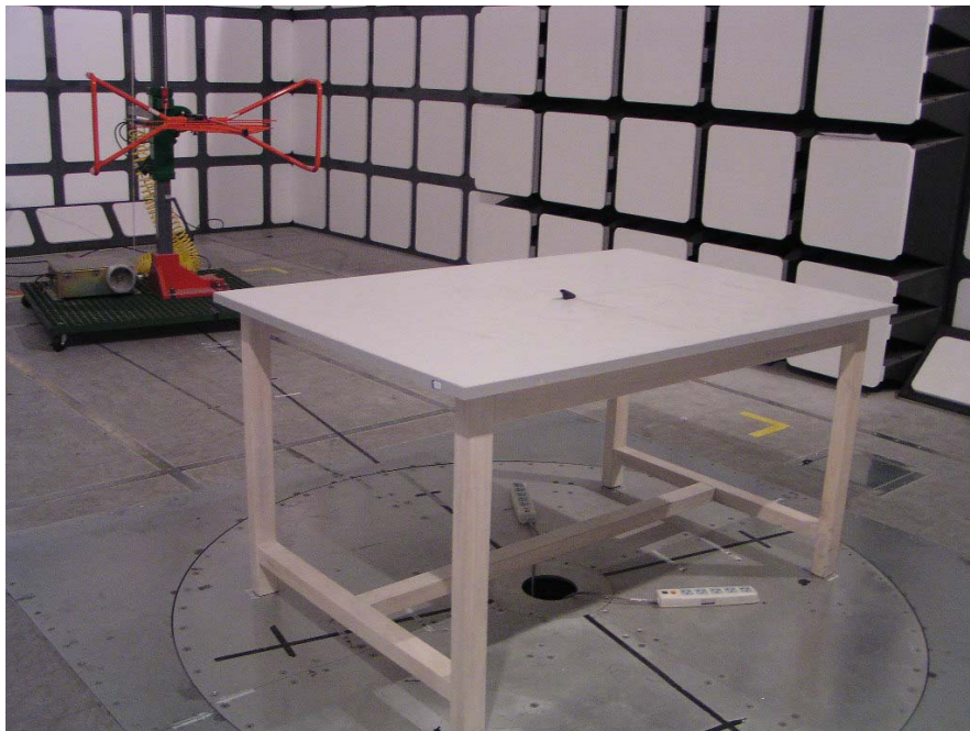
Radiated Emission - Rear View (30 MHz-1 GHz)
