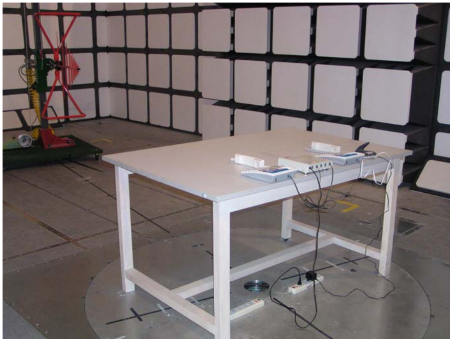
Radiated Emission - Rear View (30 MHz-1 GHz)
