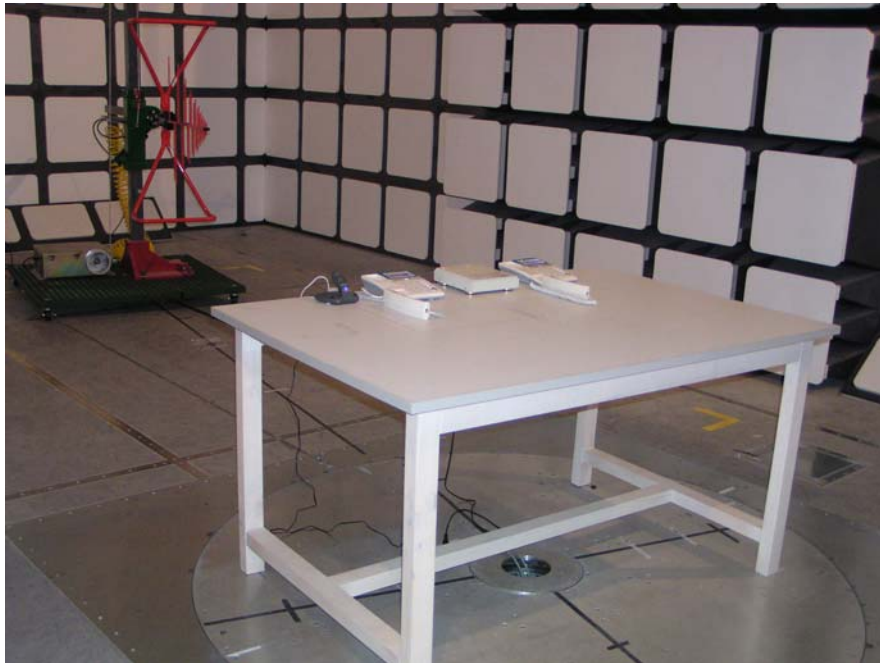
Radiated Emission - Front View (30 MHz-1 GHz)
