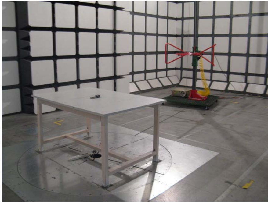
Below 1 GHz: Radiated Emissions - Front View
