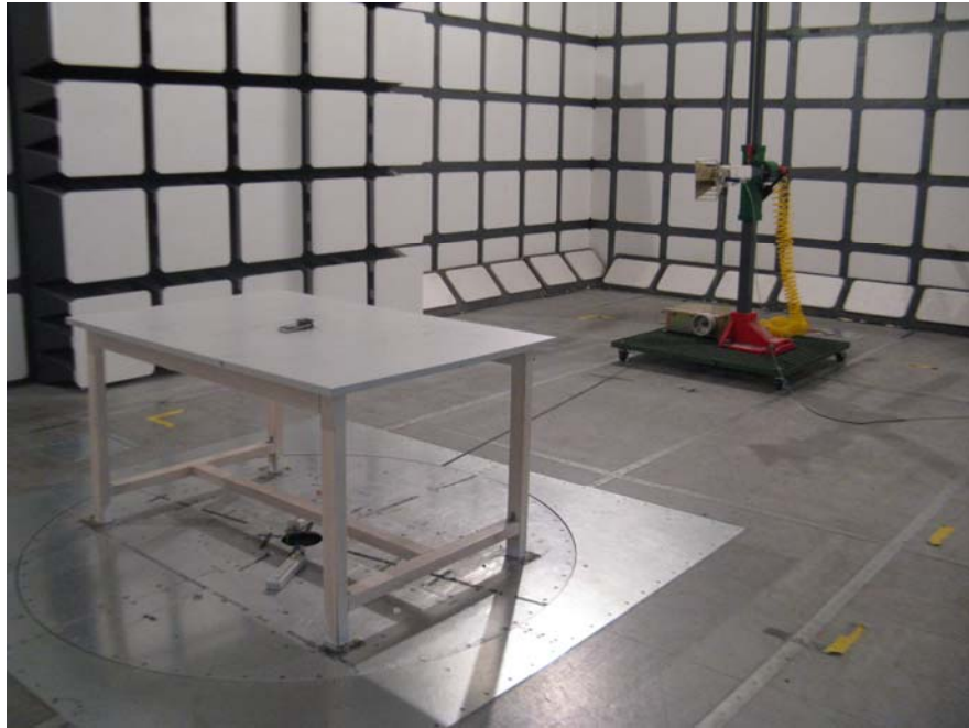
Above 1 GHz: Radiated Emissions - Rear View
