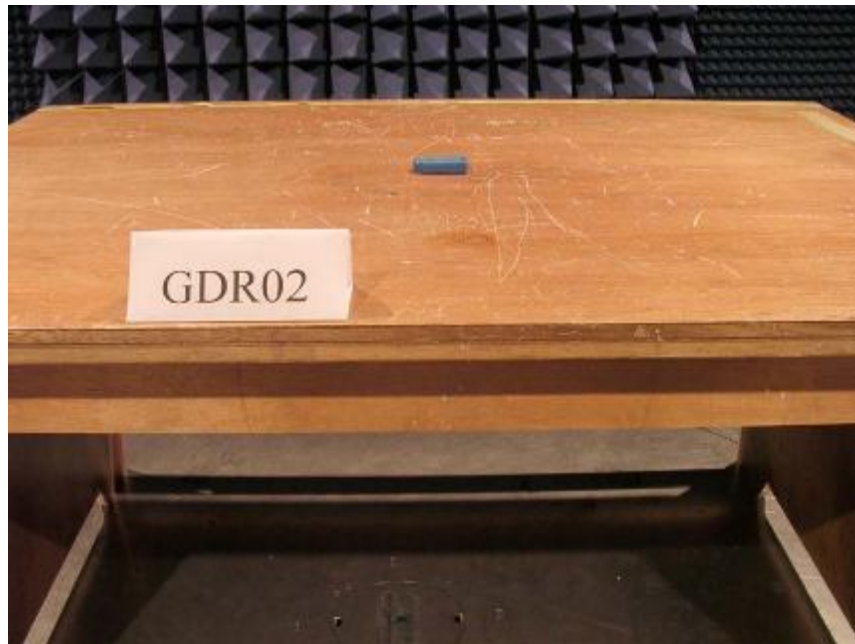
Photo 2: Radiated Emission Test Set-up
