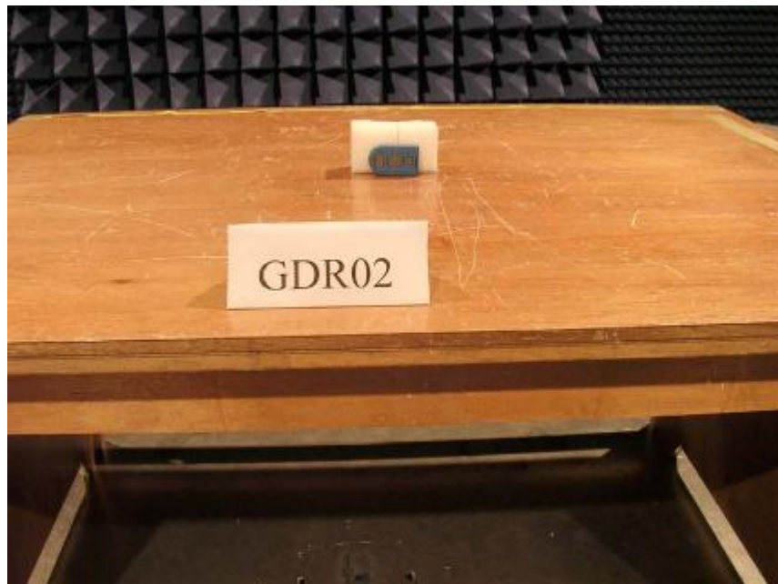
Photo 2: Radiated Emission Test Set-up
