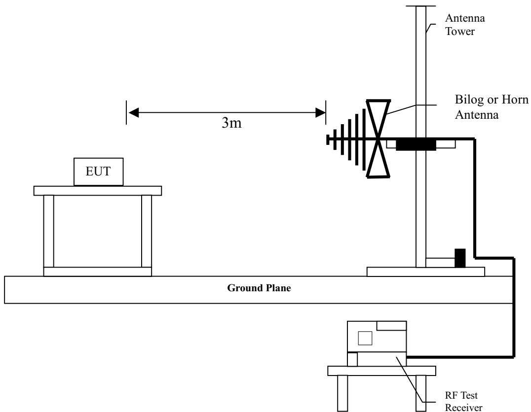
The signal is maximized through rotation and placement in the three orthogonal axes. Radiated emission measurement were performed from 30MHz to the tenth harmonic of the highest fundamental frequency.
