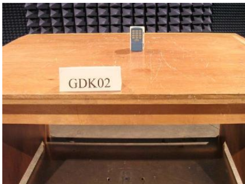
Photo 3: Radiated Emission Test Set-up
