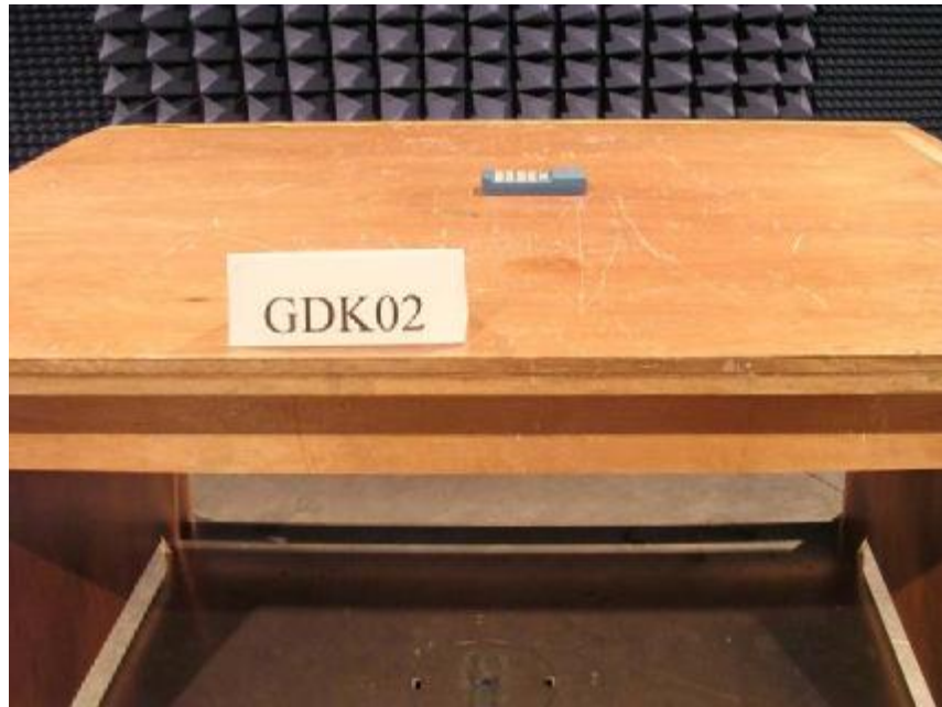
Photo 2: Radiated Emission Test Set-up
