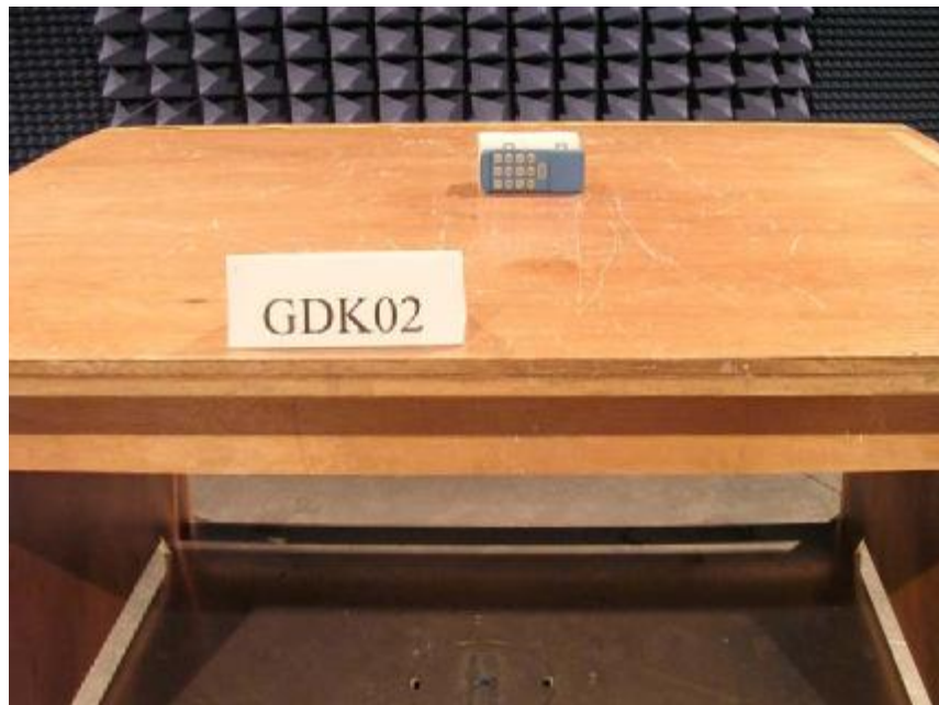
Photo 2: Radiated Emission Test Set-up
