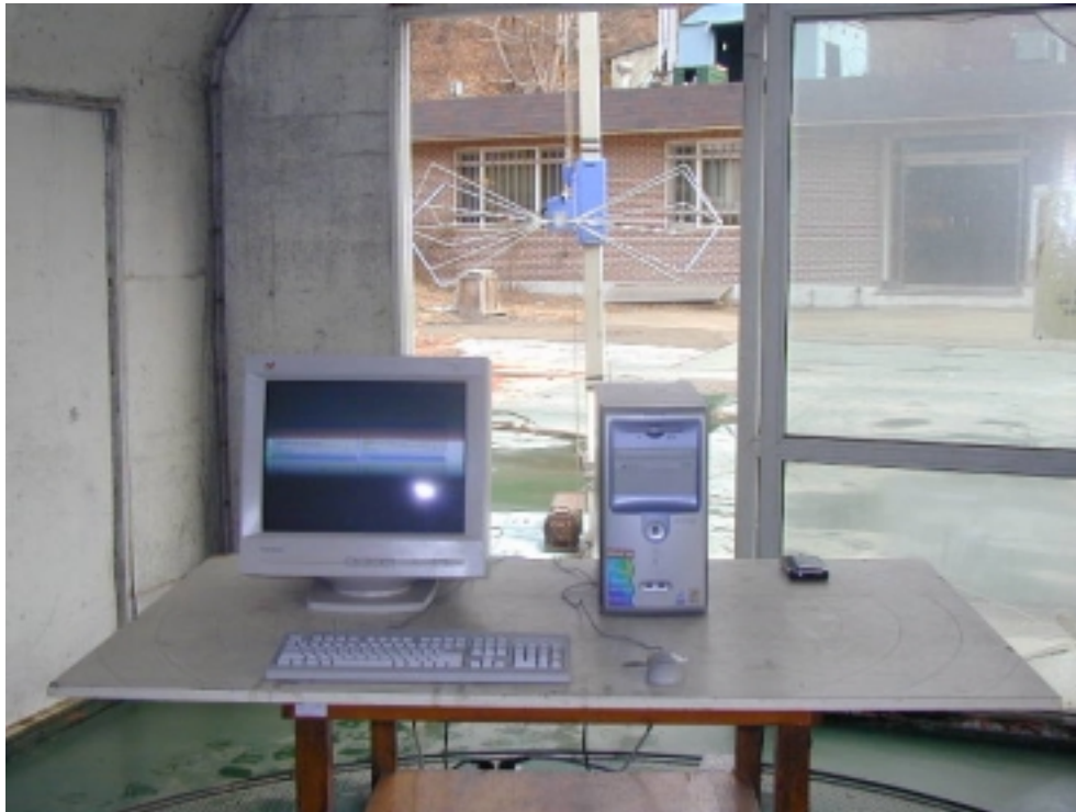
RADIATED EMISSION SETUP PHOTOGRAPH - FRONT VIEW ( 30 - 300 MHz )
