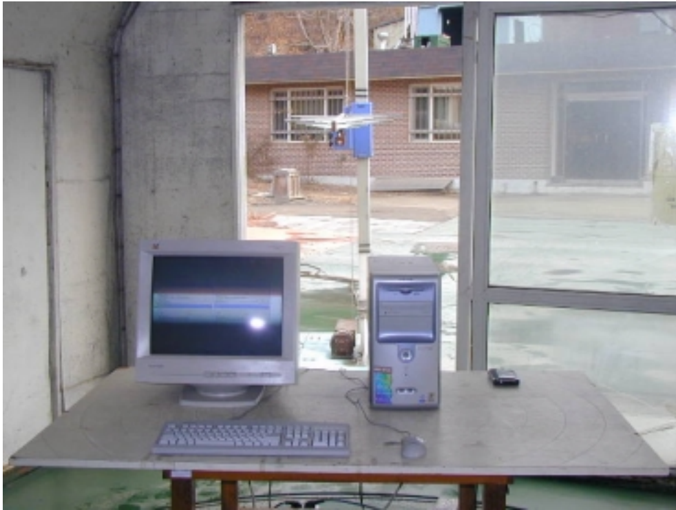
RADIATED EMISSION SETUP PHOTOGRAPH - FRONT VIEW ( 300- 1000 MHz )
