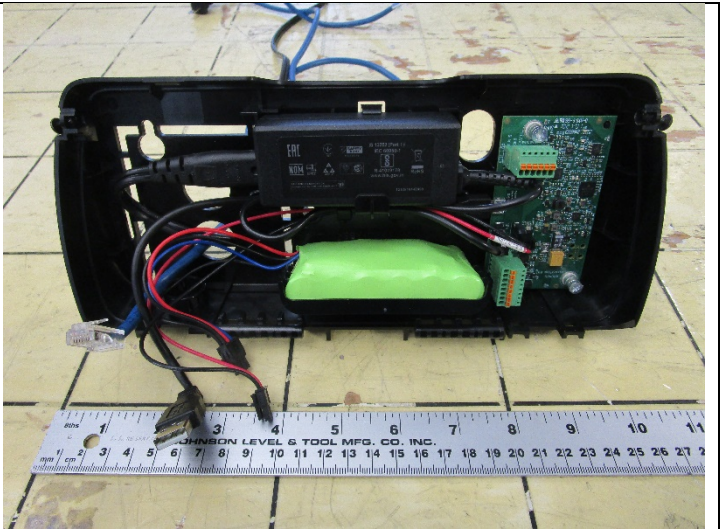
Figure 2: External Chassis Back - AC/DC Power Converter, Back-up Battery, Transition Board
