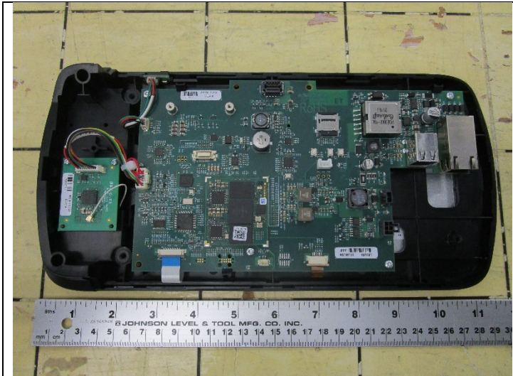
Figure 5: Internal Chassis Removed - Motherboard, Legic SmartCard Module
