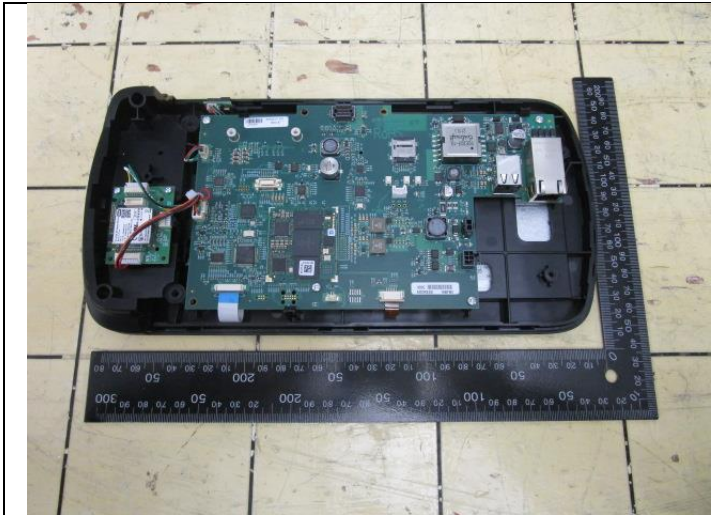
Figure 5: Internal Chassis Removed - Motherboard, HID SmartCard Module
