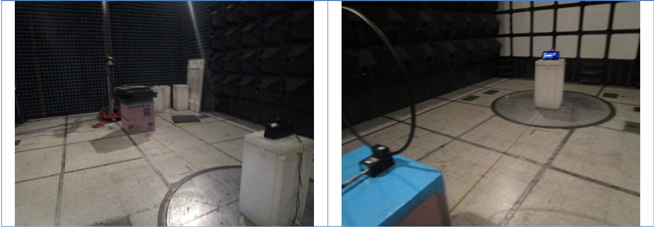
Radiated Emissions: FCC 15.209/RSS-210 | 0.009-30 MHz
