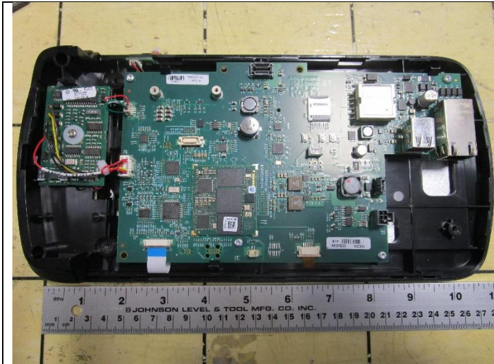
Figure 5: Internal Chassis Removed - Motherboard, HID Proximity reader
