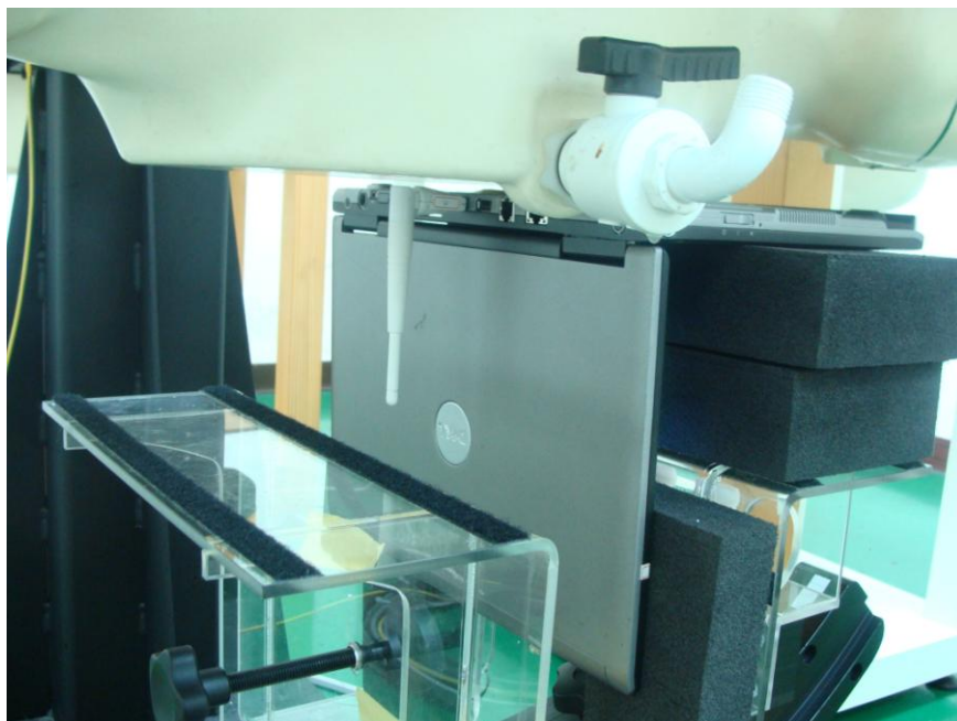
Direct laptop plug-in for USB Configuration 1 (Horizontal Up with Phantom 5 mm Gap, Antenna set Perpendicular)
