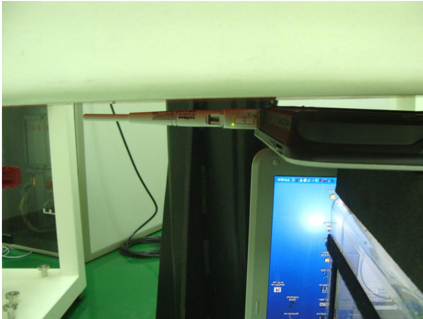
Direct laptop plug-in for USB Configuration 4 (Vertical Back with Phantom 5 mm Gap Antenna set Straight)
