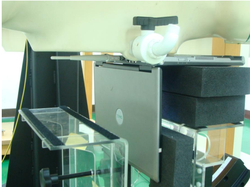
Direct laptop plug-in for USB Configuration 1 (Horizontal Up with Phantom 5 mm Gap, Antenna set Straight)
