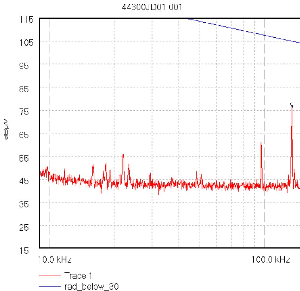
Start 9.0 kHz; Stop 150.0 kHz - Log Scale
