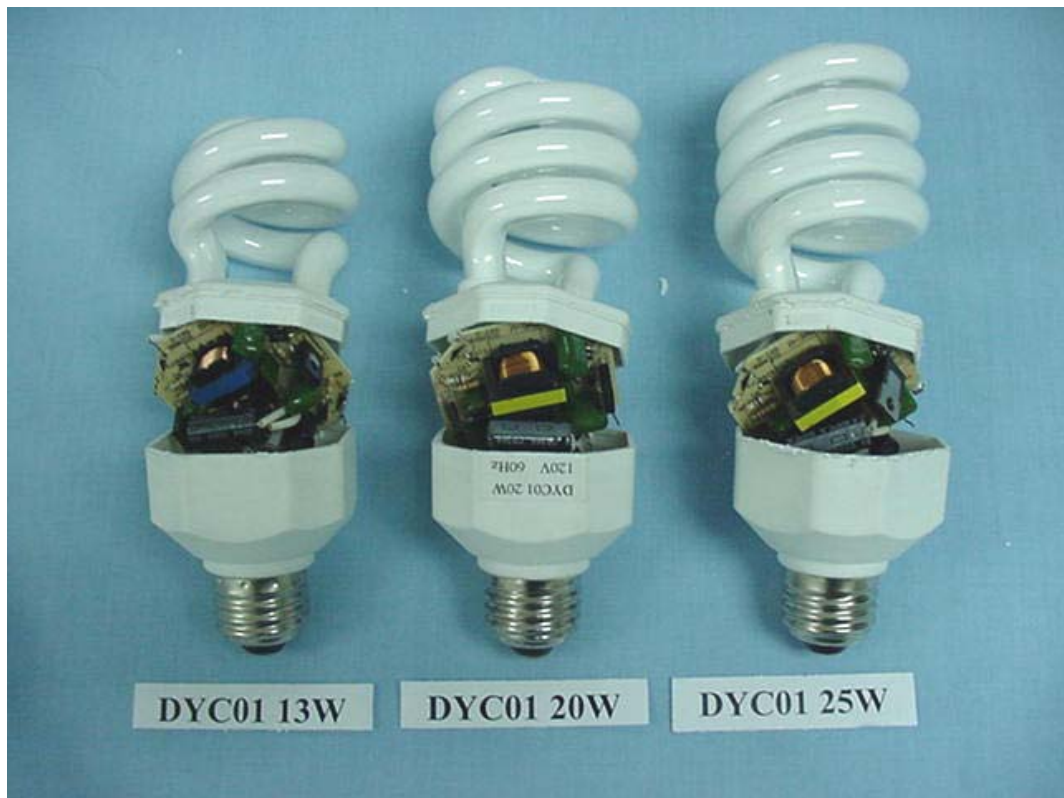
FIGURE 13 ENERGY SAVING LAMP (M/N: DYC01 13W 20W 25W) COVER REMOVED
