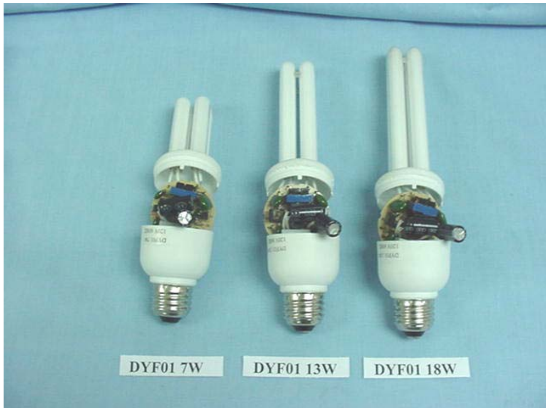
FIGURE 1 ENERGY SAVING LAMP (M/N: DYF01 7W 13W 18W) COVER REMOVED
