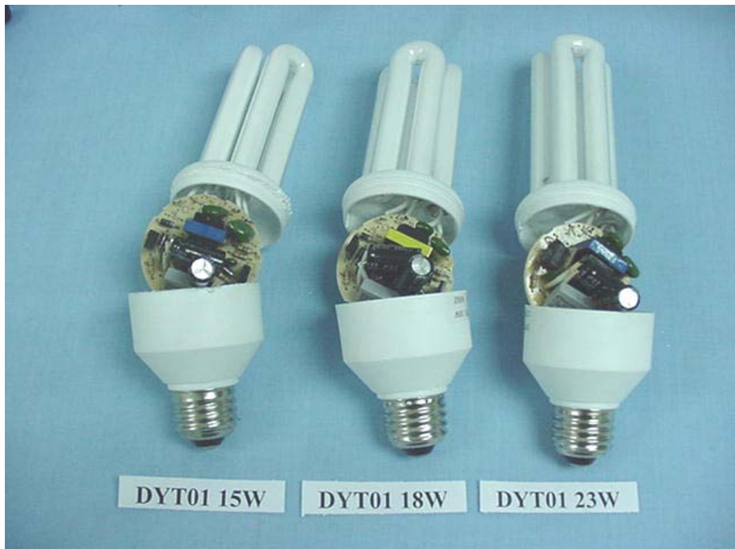
FIGURE 10 ENERGY SAVING LAMP (M/N: DYT01 15W 18W 23W) COVER REMOVED
