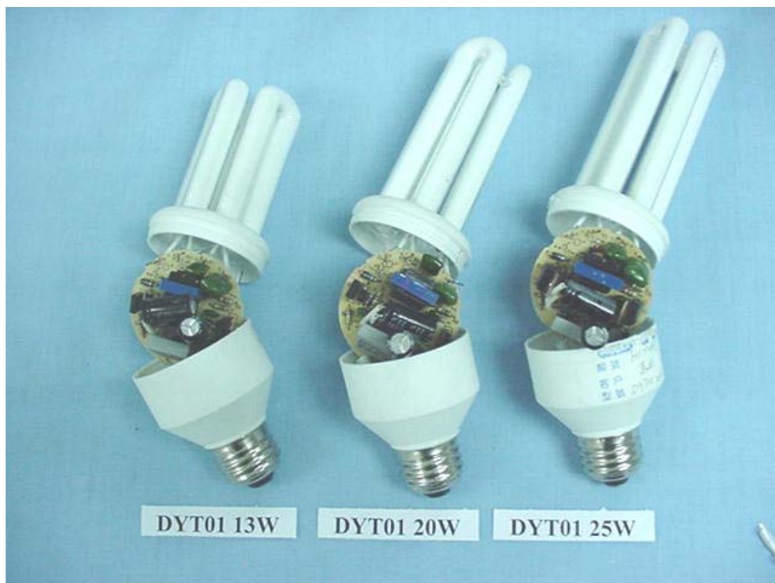
FIGURE 7 ENERGY SAVING LAMP (M/N: DYT01 13W 20W 25W) COVER REMOVED
