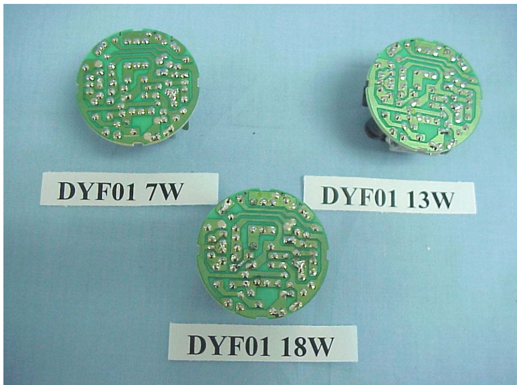
FIGURE 3 ENERGY SAVING LAMP (M/N: DYF01 7W 13W 18W) MAIN BOARD (SOLDERED SIDE)
