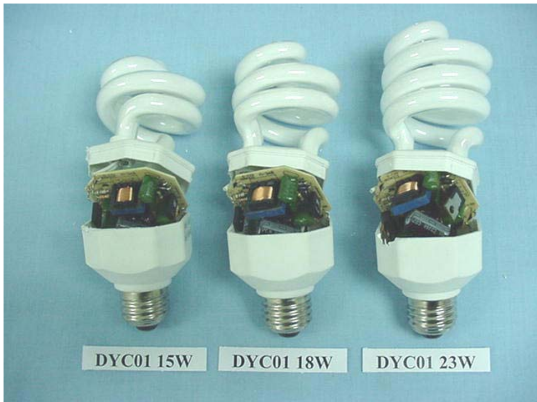
Figure 16 ENERGY SAVING LAMP (M/N: DYC01 15W 18W 23W) COVER REMOVED
