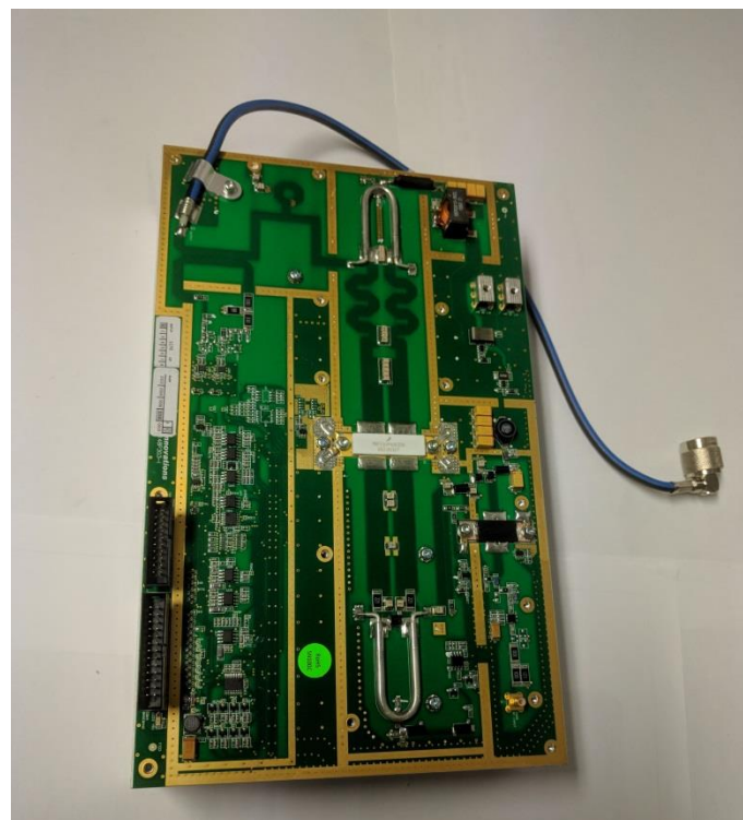
Power amplifier board top unshielded
