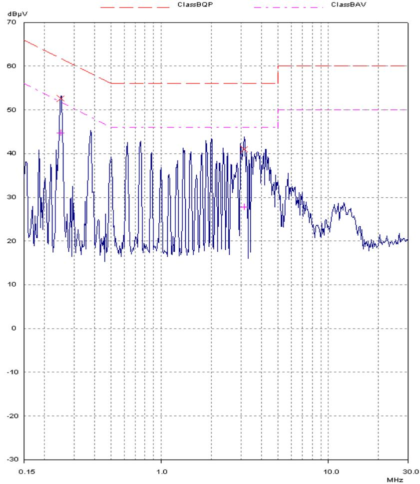
**8.2. Receiver Radiated Emission: Section 15.109**
