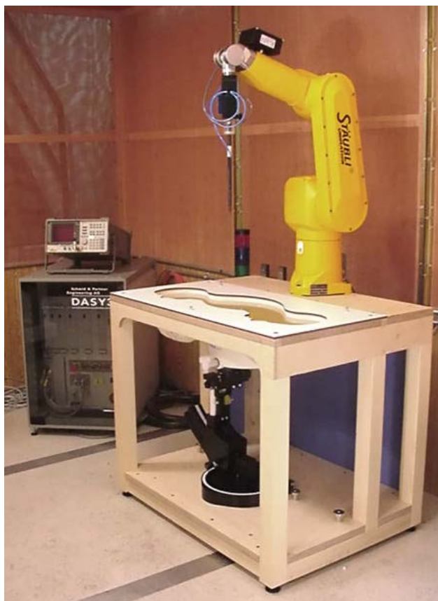
DASY3 SAR Measurement System with SAM phantom
