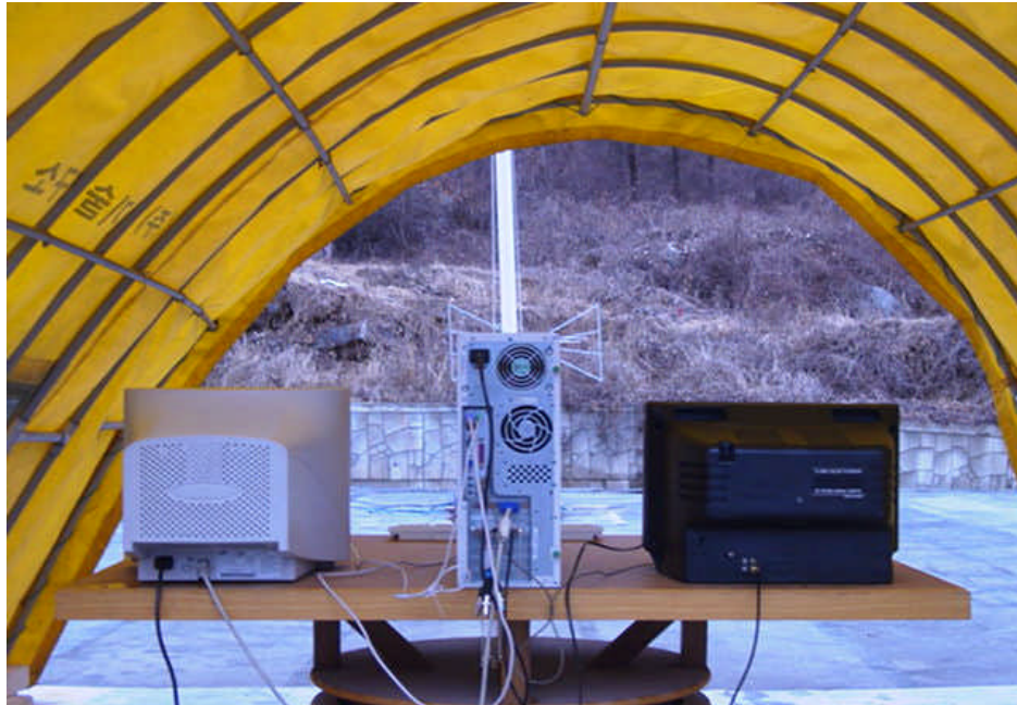
Photograph 1 : Setup for radiated Emissions
