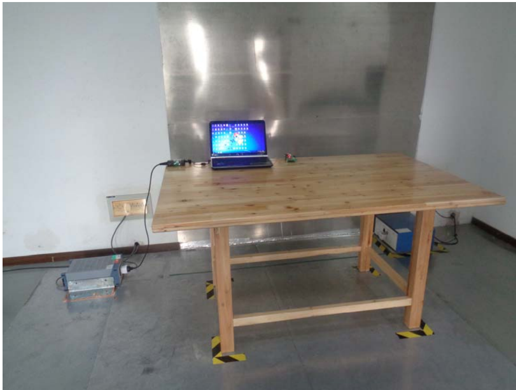
Conducted Emissions Test Setup – Front View(EMW3165-P)
