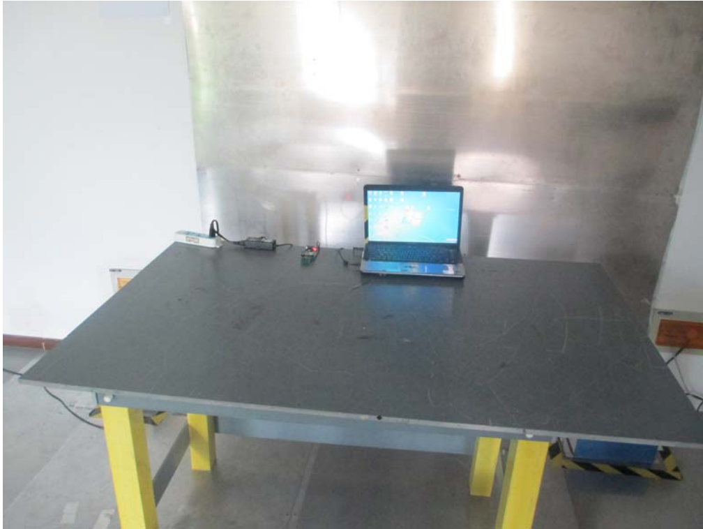
Conducted Emissions Test Setup Front View
