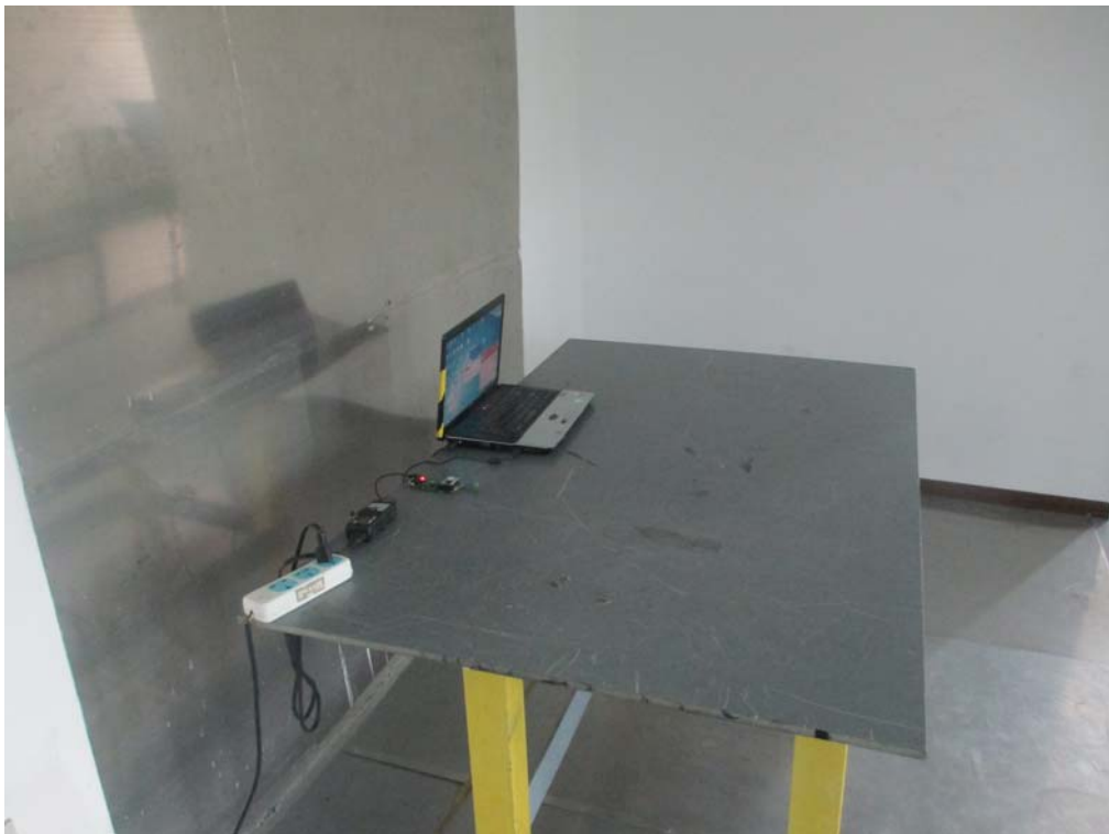
Conducted Emissions Test Setup Side View
