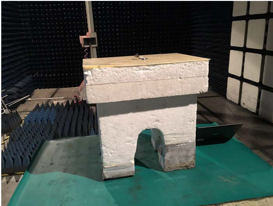
Spurious Emission Test Setup (Above 1GHz)
