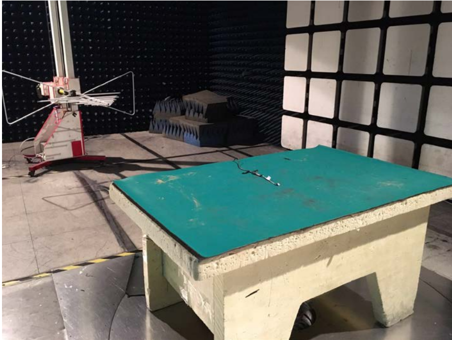
Spurious Emission Test Setup (Below 1GHz)
